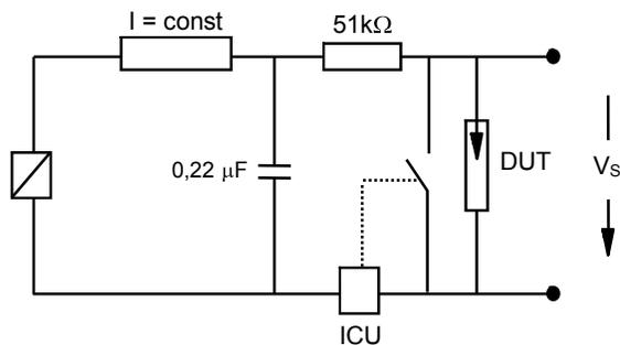
DUT device under test
