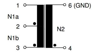
Recommendation: Connect Pin 6 on PCB to GND
