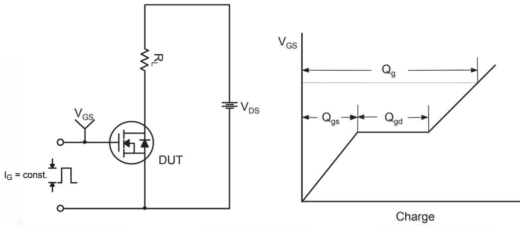
Fig 13. Gate Charge Test Circuit & Waveform
