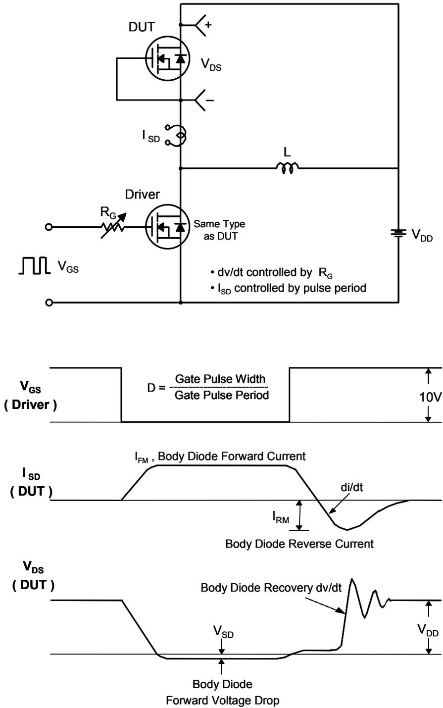
Fig 16. Peak Diode Recovery  $dv/dt$  Test Circuit & Waveforms
