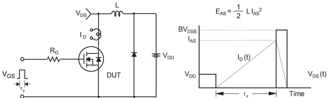
Fig 15. Unclamped Inductive Switching Test Circuit & Waveforms
