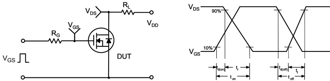
Fig 14. Resistive Switching Test Circuit & Waveforms
