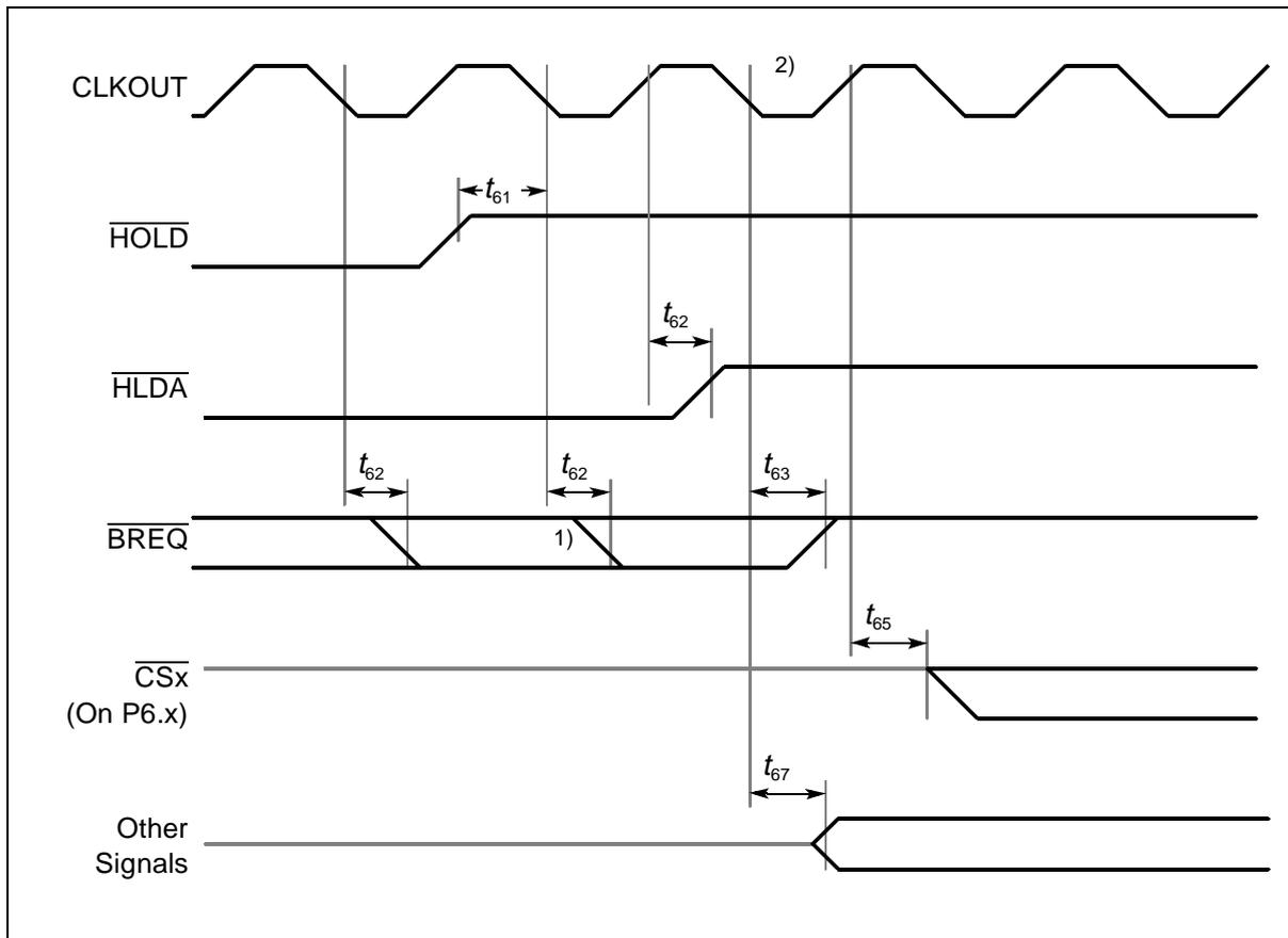
Figure 26 External bus arbitration, (regaining the bus)
