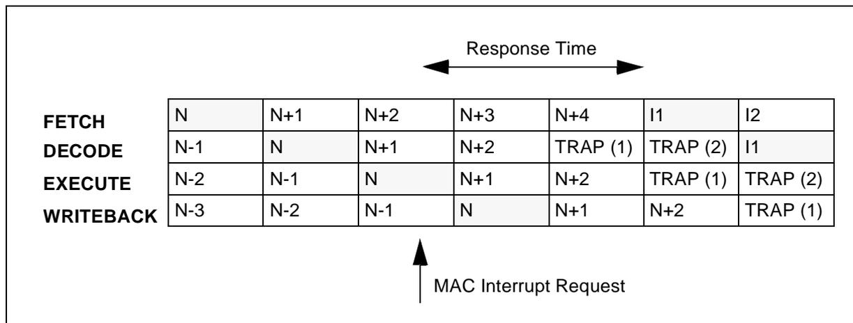
**Figure 7 Pipeline diagram for MAC interrupt response time**
