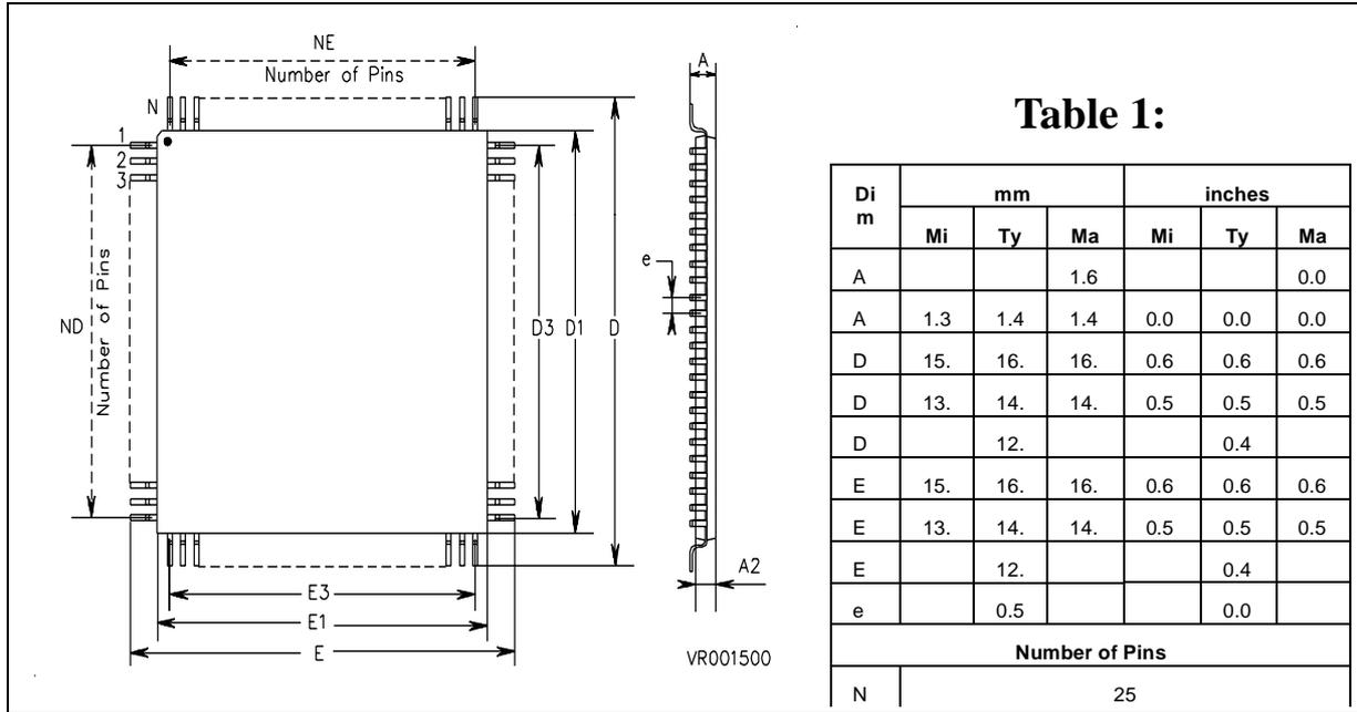
Figure 31 Package outline TQFP100 (14 x 14 mm)
