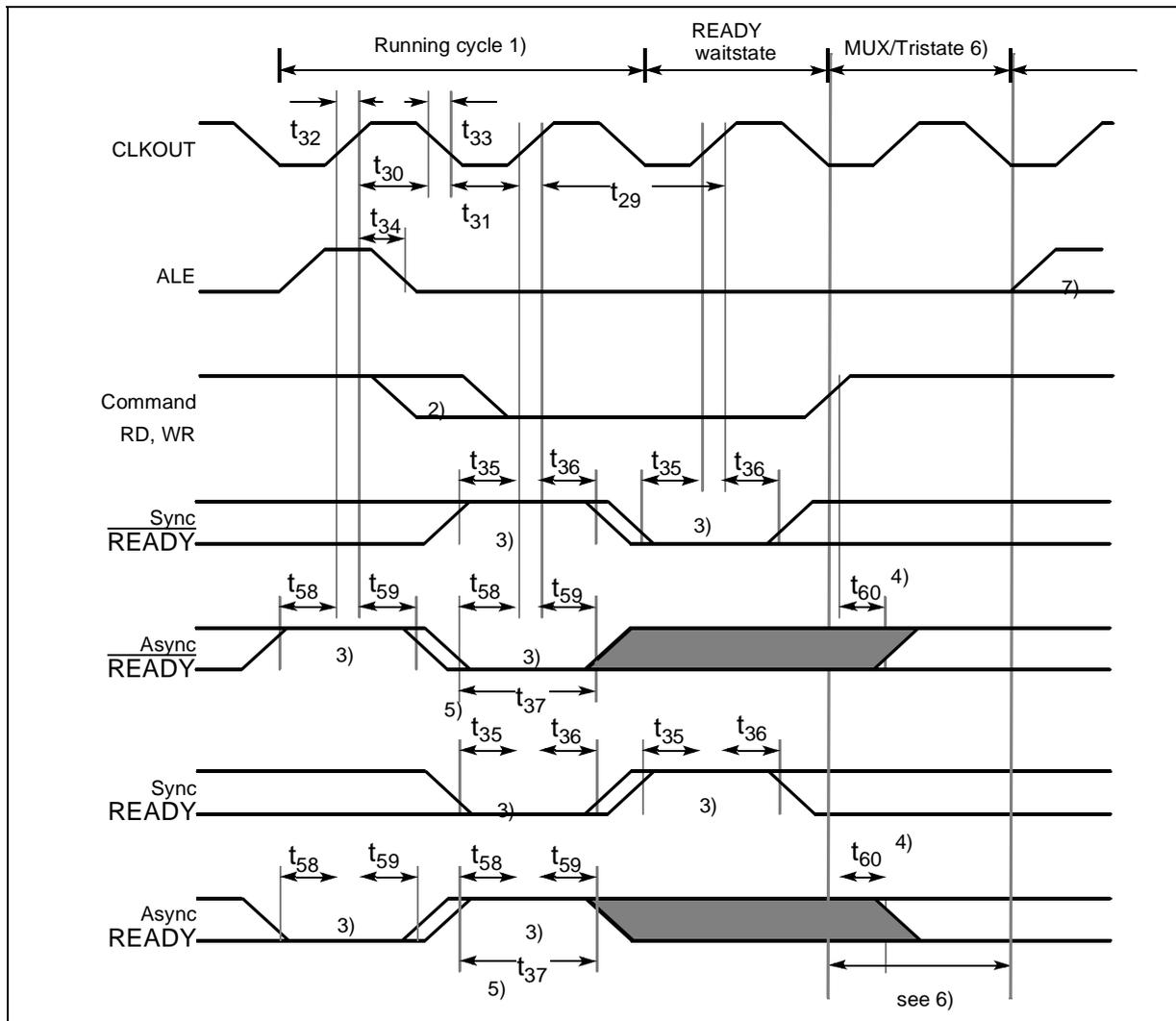
Figure 24 CLKOUT and  $\overline{\text{READY}}/\text{READY}$
