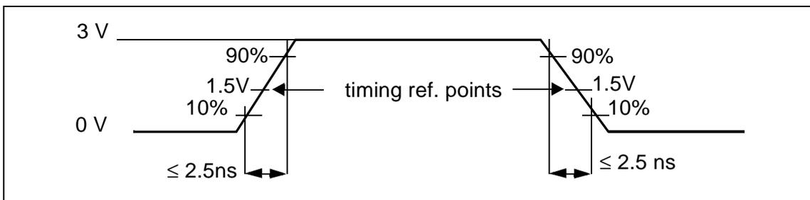
Figure 11 Input waveforms
