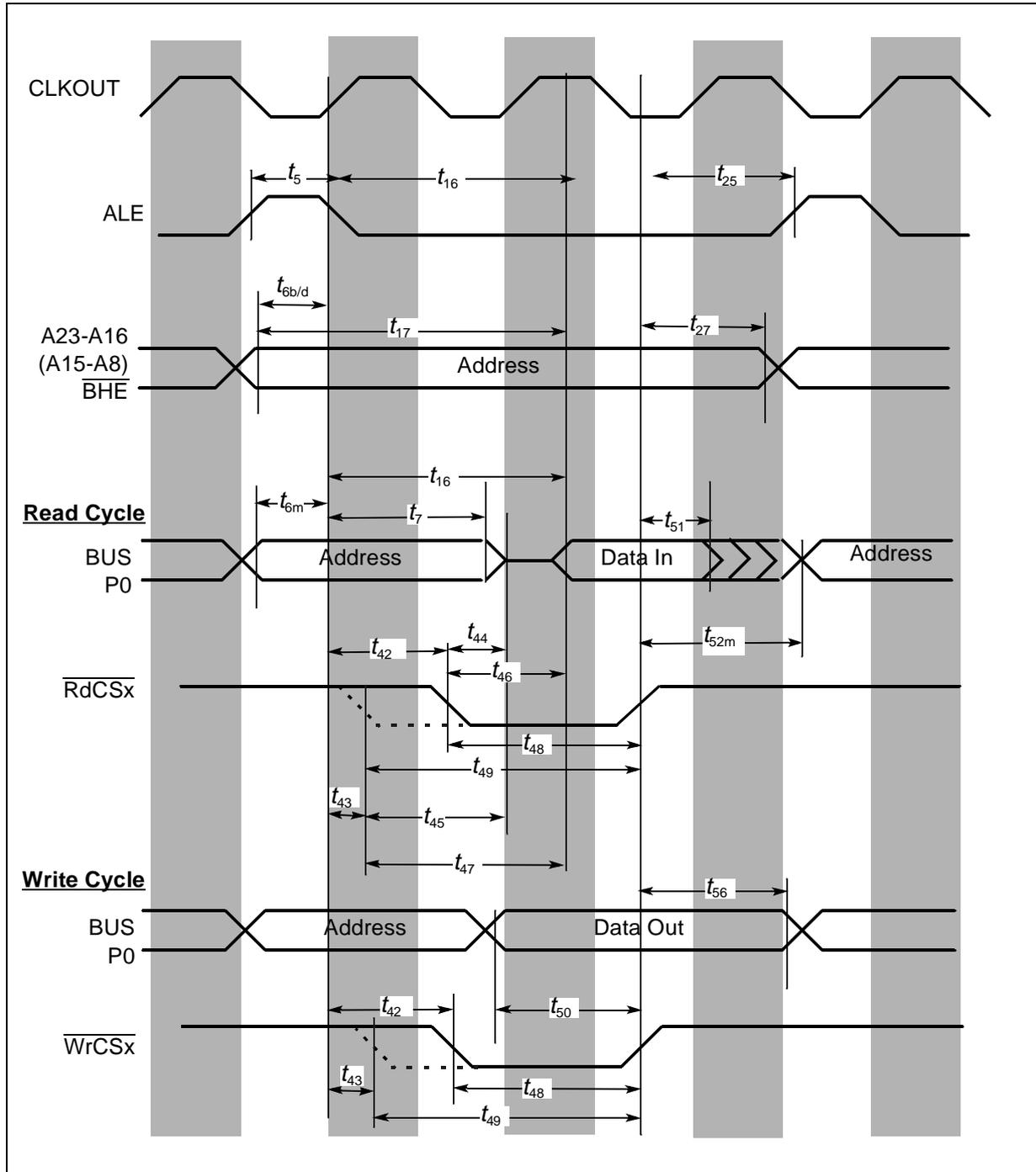
Figure 18 External memory cycle: multiplexed bus, with/without read/write delay, normal ALE, read/write chip select
