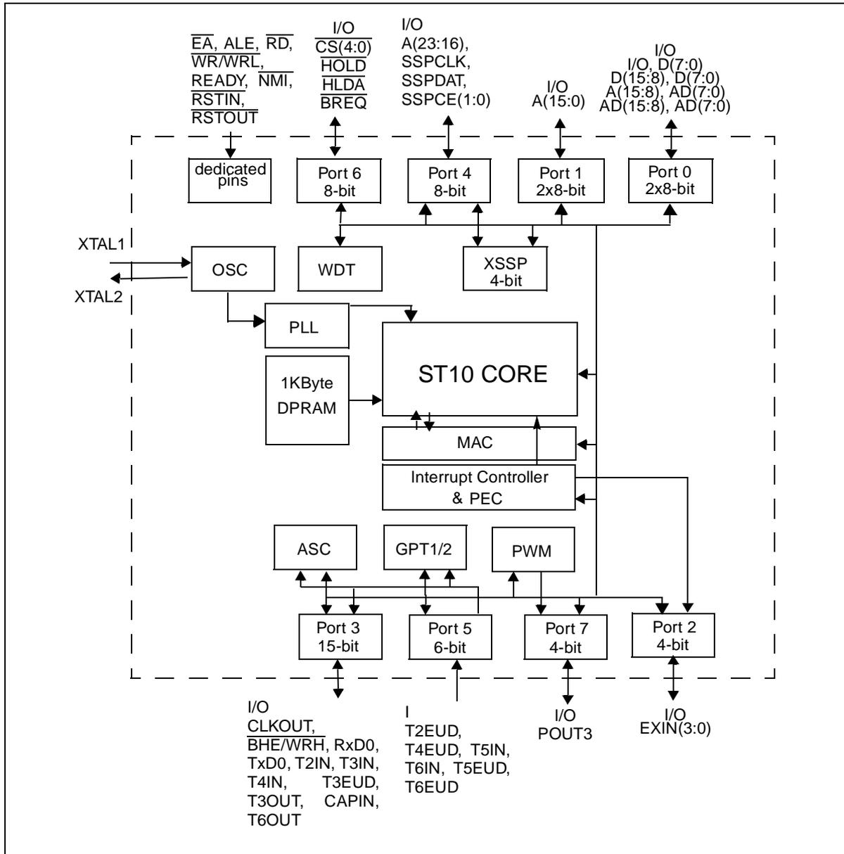
Figure 2 Block diagram
