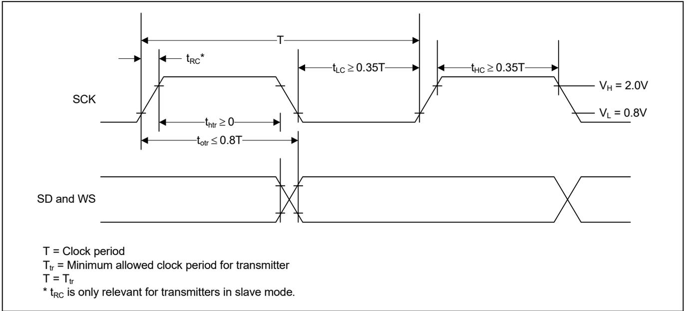
**Figure 15 I<sup>2</sup>S transmitter timing**
