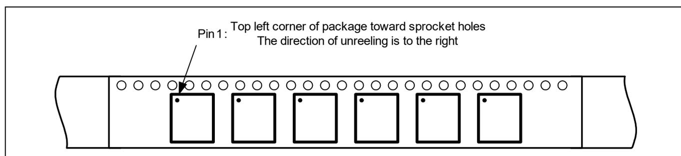
**Figure 18** Pin 1 orientation
