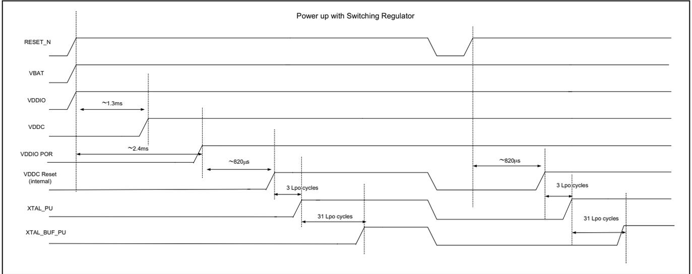
**Figure 4** Reset timing
