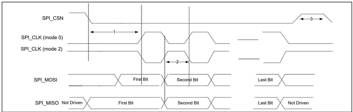
**Figure 12 SPI timing, mode 0 and 2**
