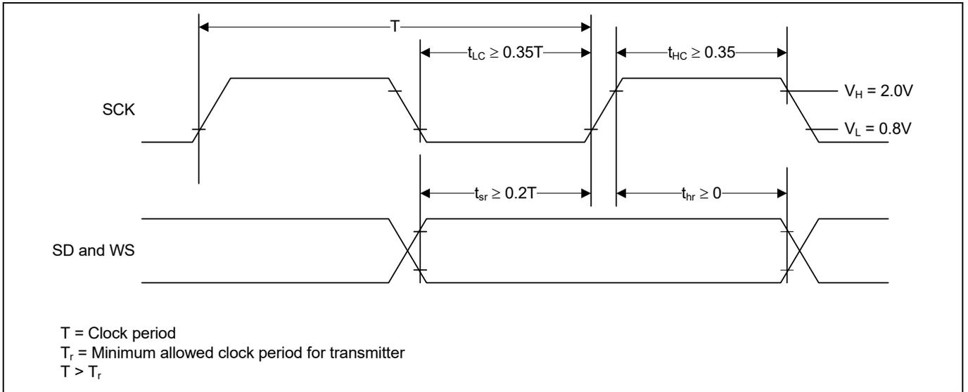
**Figure 16 I<sup>2</sup>S receiver timing**
