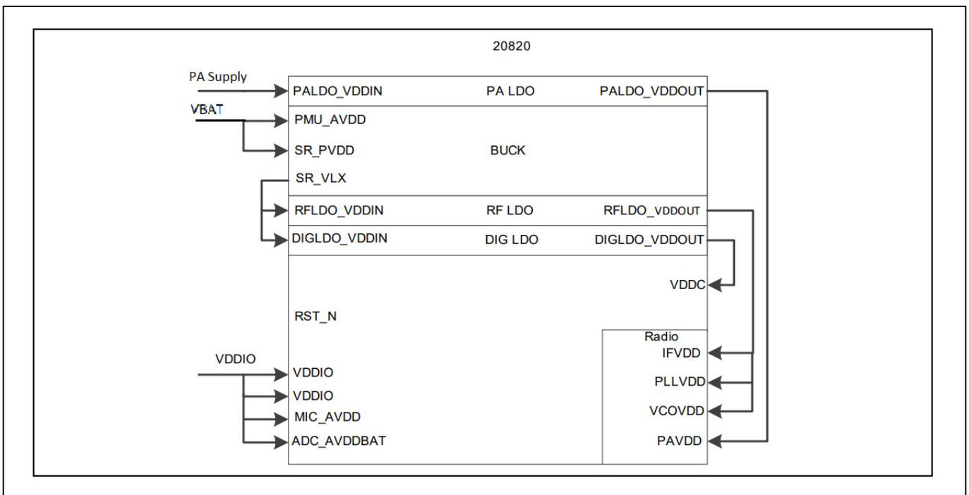
**Figure 6 Configuration 1 - VBAT and VDDIO**
