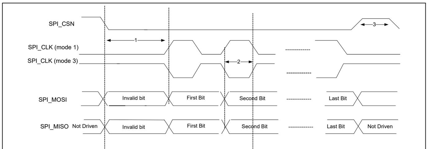
**Figure 13 SPI timing, mode 1 and 3**
