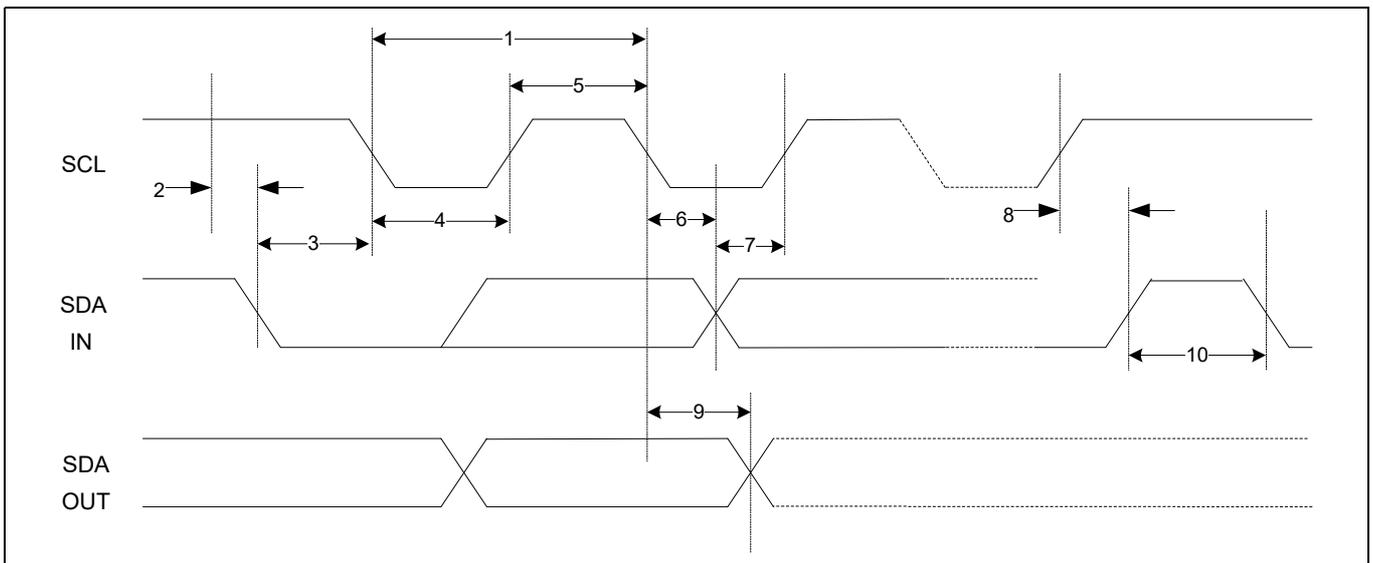
**Figure 14 I<sup>2</sup>C interface timing diagram**
