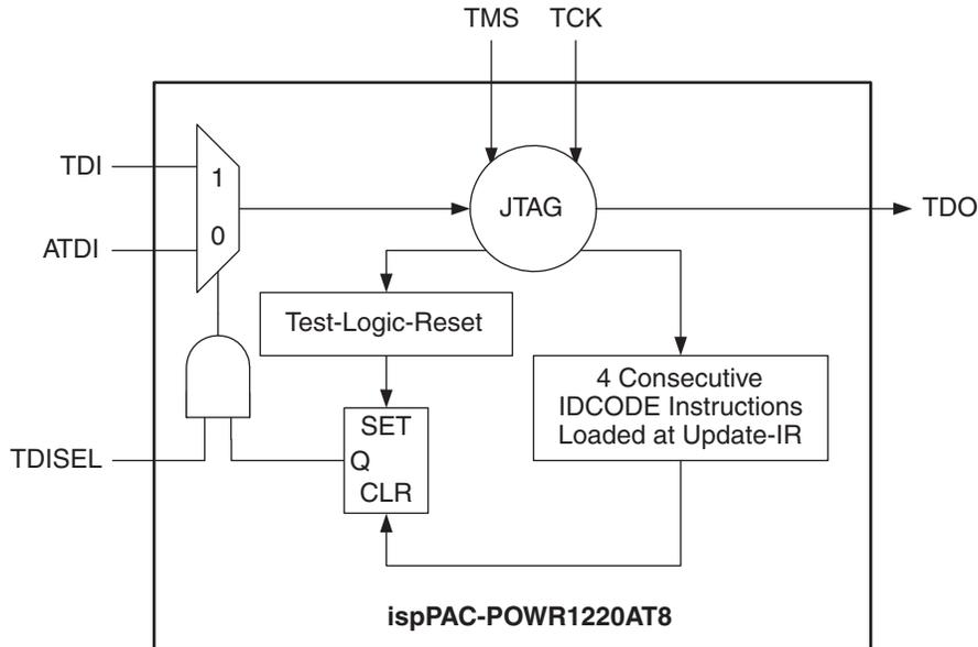
Table 12 shows in truth table form the same conditions required to select either TDI or ATDI as in the logic diagram found in Figure 36.
