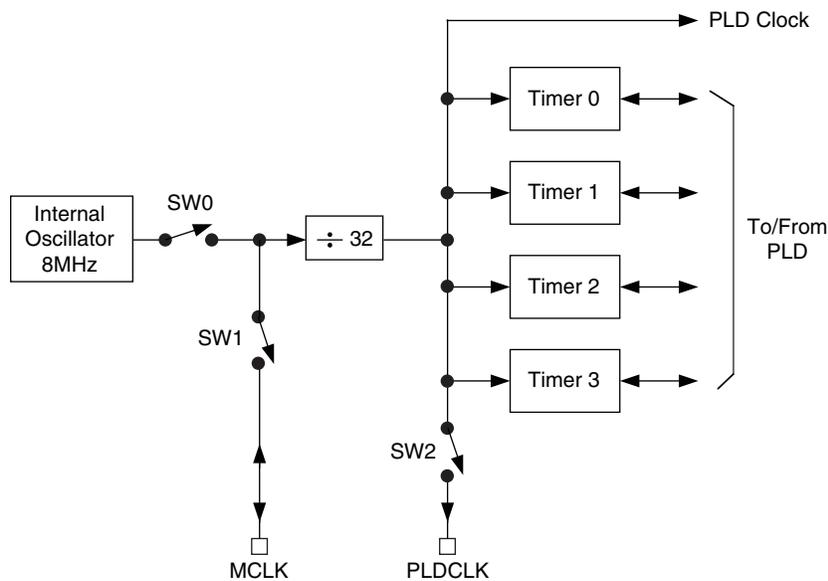
The internal oscillator runs at a fixed frequency of 8 MHz. This signal is used as a source for the PLD and timer clocks. It is also used for clocking the comparator outputs and clocking the digital filters in the voltage monitor circuits, ADC and trim circuits. The ispPAC-POWR1220AT8 can be programmed to operate in three modes: Master
