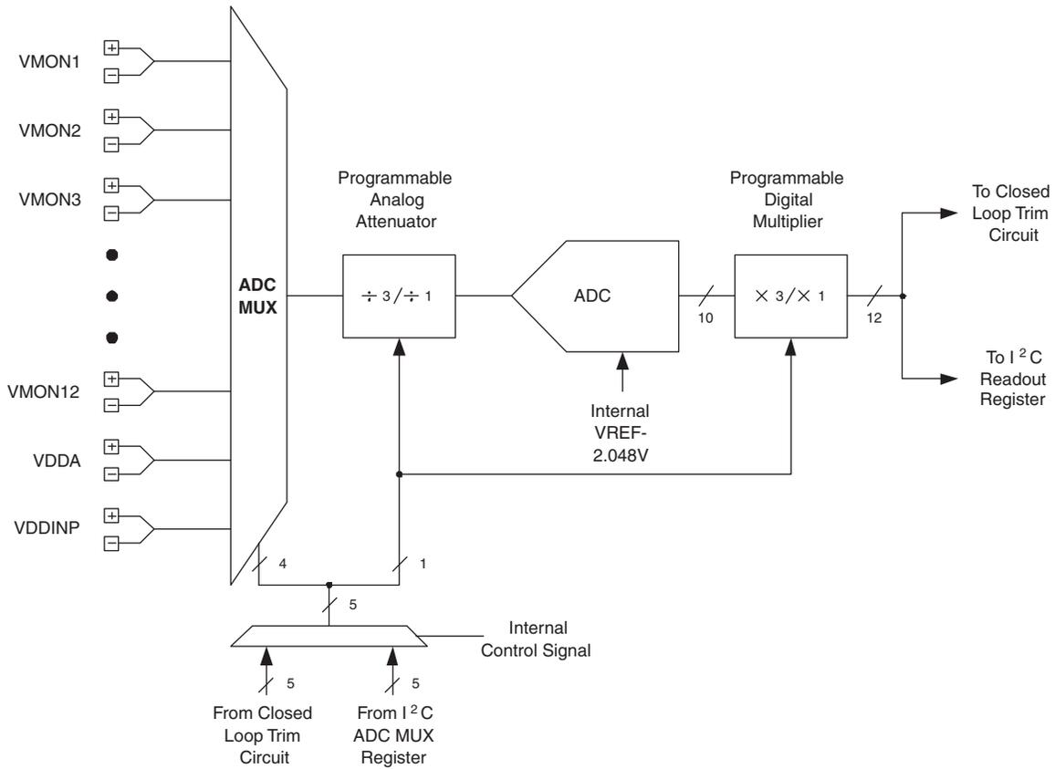
Figure 9 shows the ADC circuit arrangement within the ispPAC-POWR1220AT8 device. The ADC can measure all analog input voltages through the multiplexer, ADC MUX. The programmable attenuator between the ADC mux and the ADC can be configured as divided-by-3 or divided-by-1 (no attenuation). The divided-by-3 setting is used to measure voltages from 0V to 6V range and divided-by-1 setting is used to measure the voltages from 0V to 2V range.
