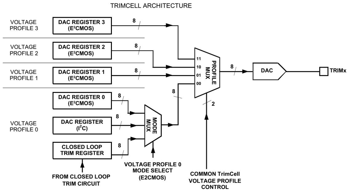
Figure 15 shows four power supply voltages next to each DC-DC converter. When the Profile MUX is set to Voltage Profile 3, the DC supply controlled by Trim 1 will be at 0.95V, the DC supply controlled by Trim 2 will be at 1.14V, 1.43V for Trim 3 and 3.14V for Trim 8. When Voltage Profile 0 is selected, Trim 1 will set the supply to 1V, Trim 2 and Trim 3 will be set by the values that have been loaded using I<sup>2</sup>C at 1.2 and 1.5V, and Trim 8 will be set to 3.3V.
