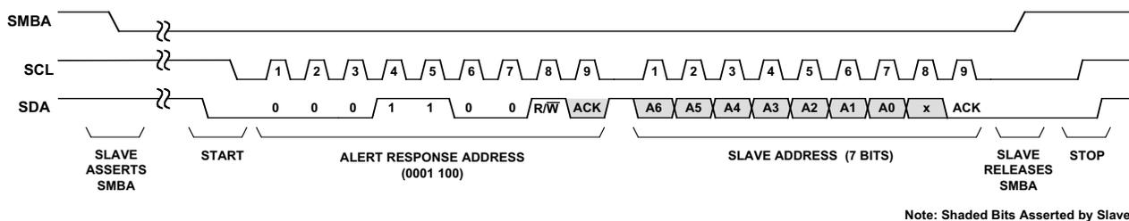
After OUT5/SMBA has been released, the bus master (typically a microcontroller) may opt to perform some service functions in which it may send data to or read data from the ispPAC-POWR1220AT8. As part of the service functions, the bus master will typically need to clear whatever condition initiated the SMBAlert request, and will also need to reset GP5\_ENb to re-enable the SMBAlert function. For further information on the SMBus, the user should consult the SMBus Standard.
