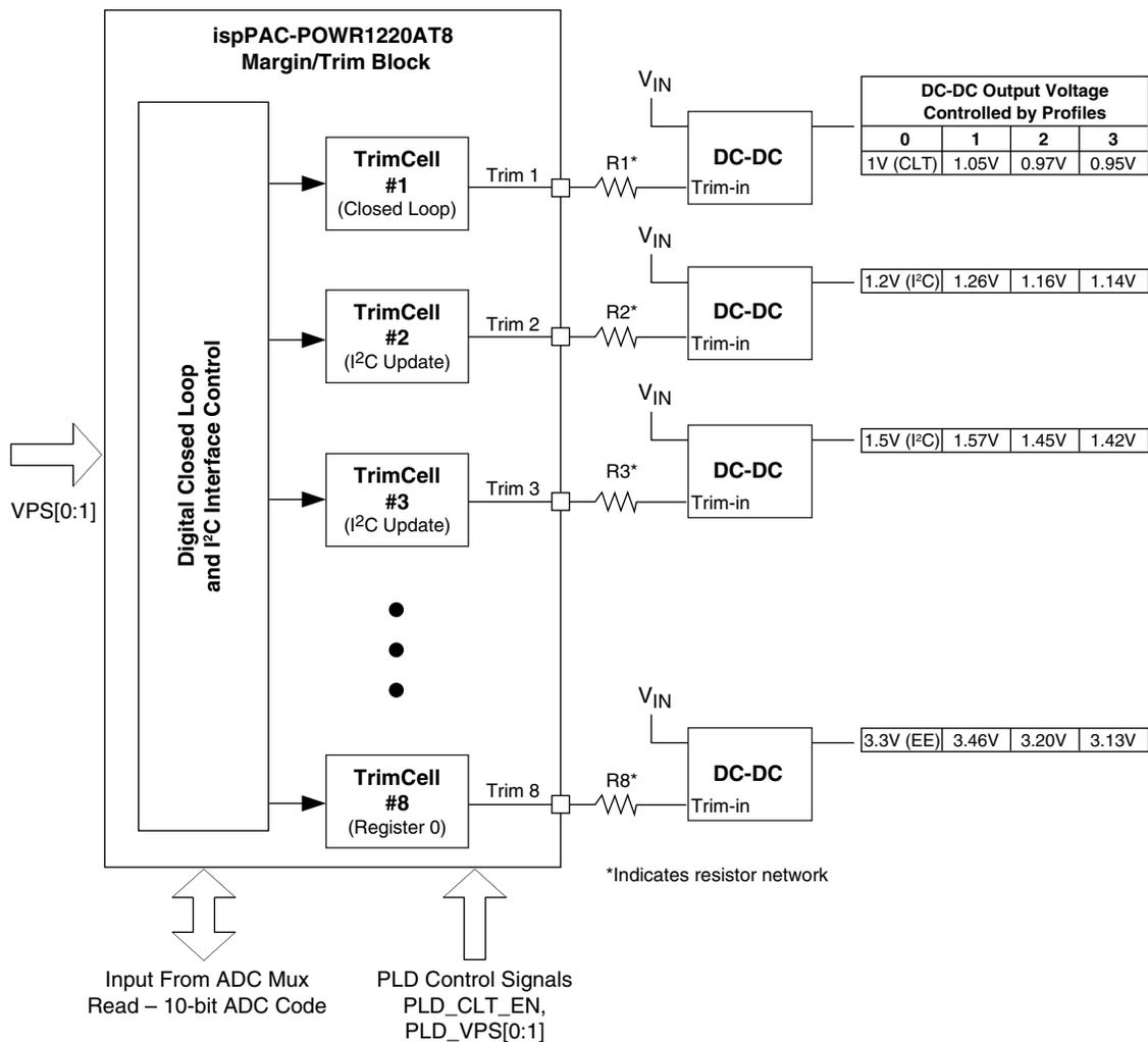
There are eight TrimCells in the ispPAC-POWR1220AT8 device, enabling simultaneous control of up to eight individual power supplies. Each TrimCell can generate up to four trimming voltages to control the output voltage of the DC-DC converter.
