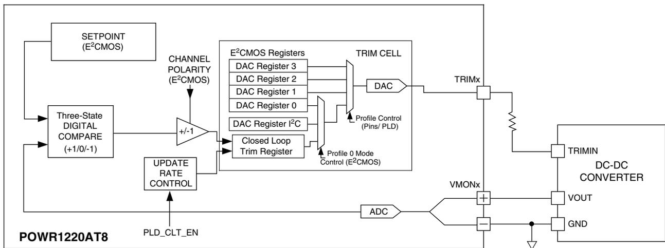
The closed loop trim cycle interval is programmable and is set by the update rate control register. The following table lists the programmable update interval that can be selected by the update rate register.
