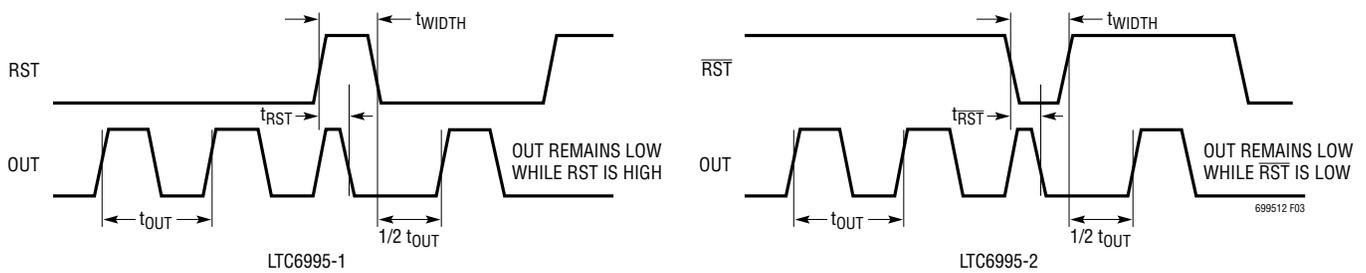
Figure 3. Reset Timing Diagram (POL Bit = 0)
