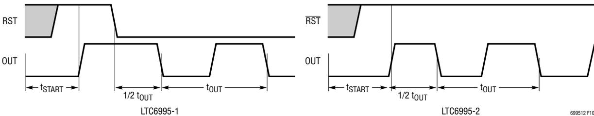
Figure 10. Start-Up Timing Diagram (Reset = 1, POL Bit = 1)
