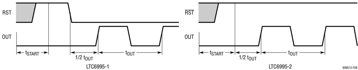
Figure 8. Start-Up Timing Diagram (Reset = 1, POL Bit = 0)
