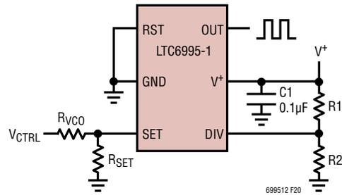
Figure 20. Voltage-Controlled Oscillator
