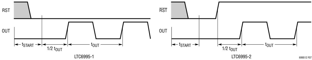
Figure 7. Start-Up Timing Diagram (Reset = 0, POL Bit = 0)
