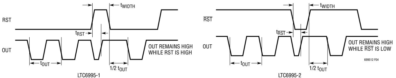
Figure 4. Reset Timing Diagram (POL Bit = 1)
