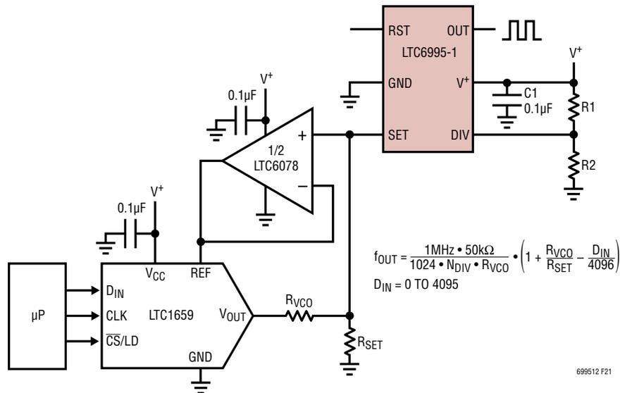
Figure 21. Digitally-Controlled Oscillator
