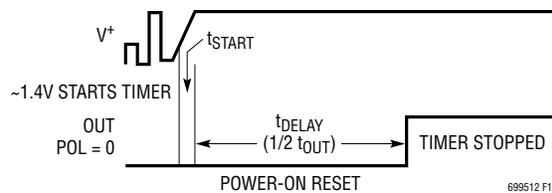
**Figure 12. Active Low Power-On Reset (1 Second Interval Example)**
