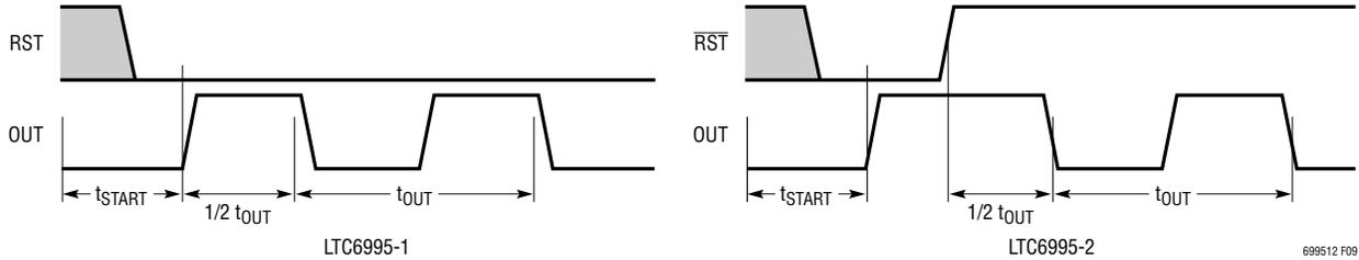
Figure 9. Start-Up Timing Diagram (Reset = 0, POL Bit = 1)
