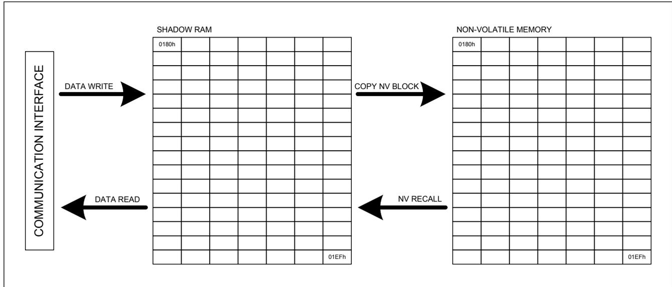
Figure 25. Shadow RAM and Nonvolatile Memory Relationship
