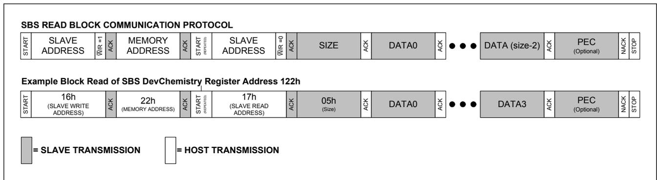
Figure 38. Example SBS Read Block Communication Sequence
