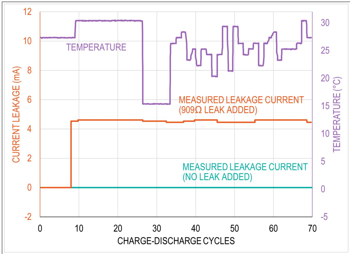
Figure 9. Example of Internal Self-Discharge with Temperature Variation
