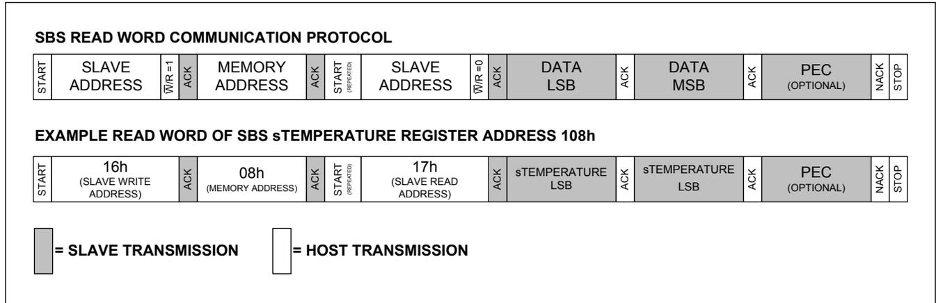
Figure 37. Example SBS Read Word Communication Sequence
