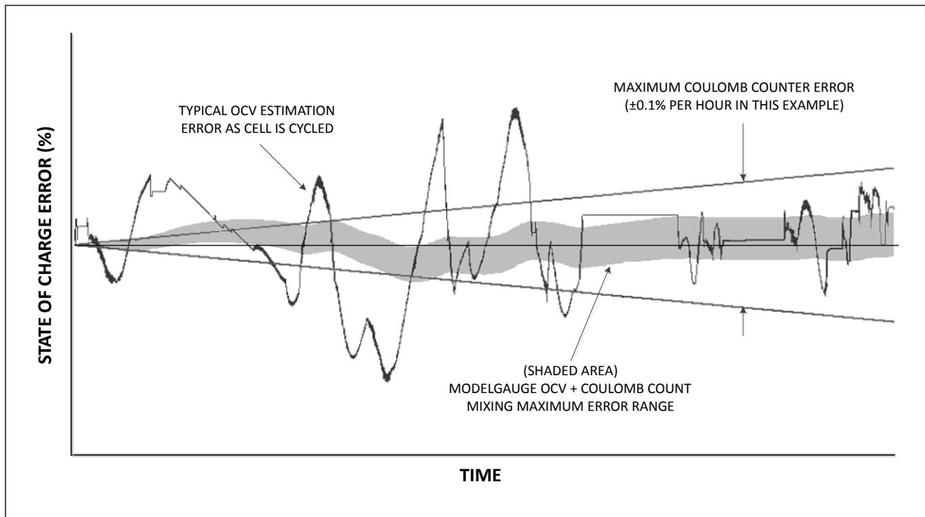
Figure 17. ModelGauge m5 EZ Typical Accuracy Example
