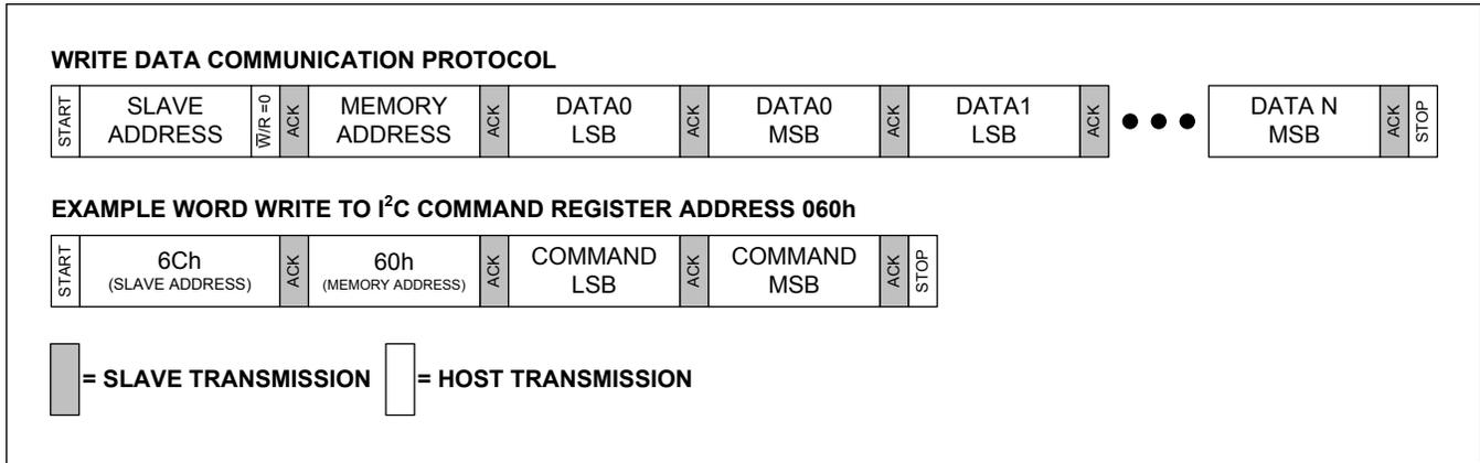
Figure 34. Example I<sup>2</sup>C Write Data Communication Sequence
