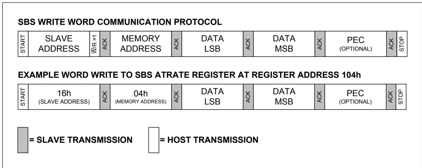
Figure 36. Example SBS Write Word Communication Sequence
