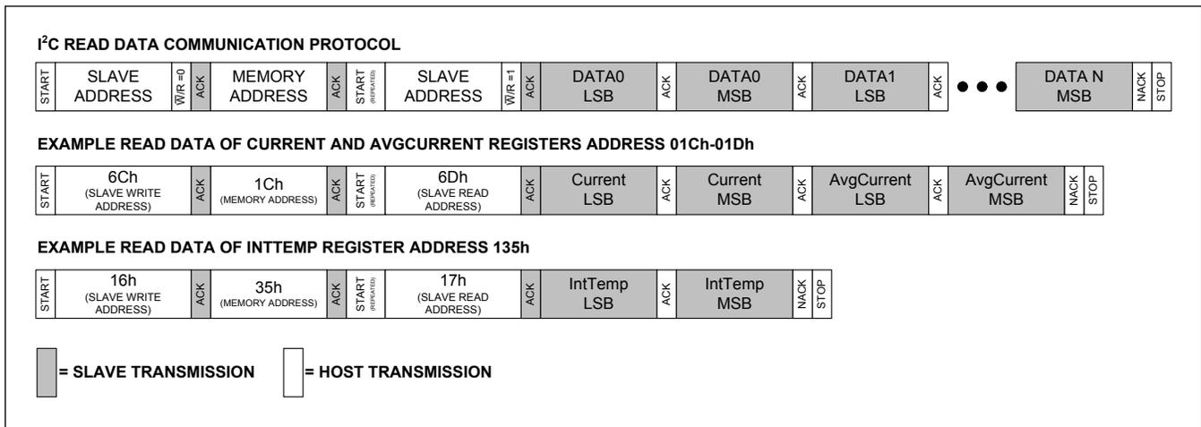
Figure 35. Example I<sup>2</sup>C Read Data Communication Sequence
