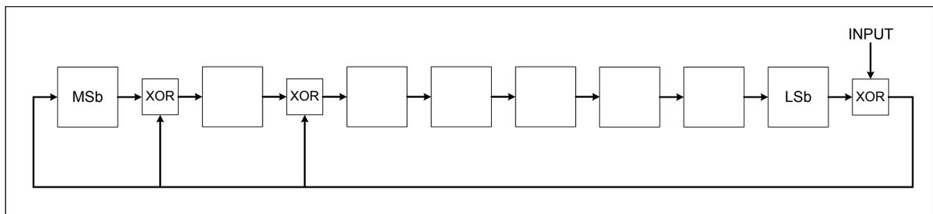
*Figure 39. PEC CRC Generation Block Diagram***Appendix A: Reading History Data Pseudo-Code Example**
