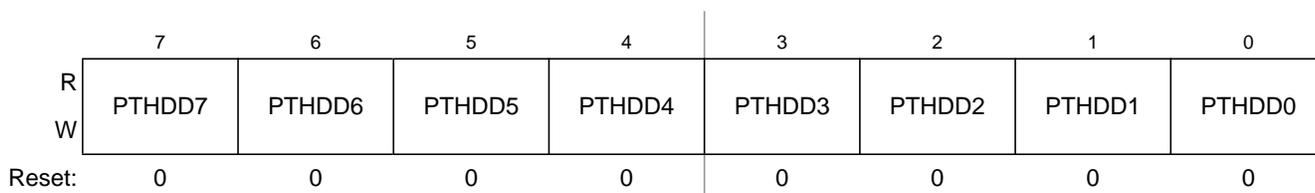
Figure 6-45. Port H Data Direction Register (PTHDD)
