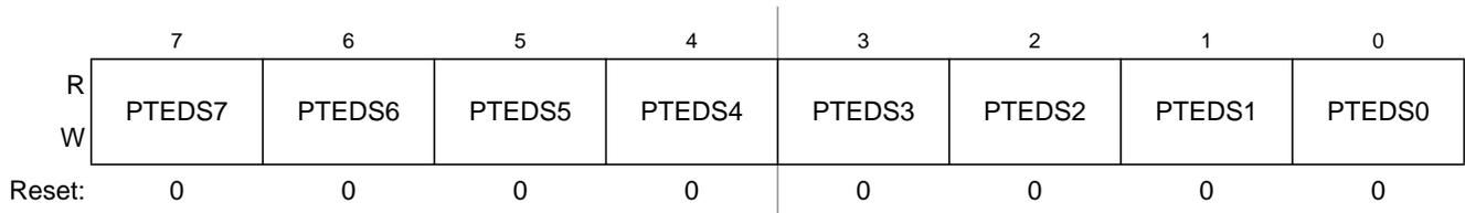
Figure 6-33. Drive Strength Selection for Port E Register (PTEDS)
