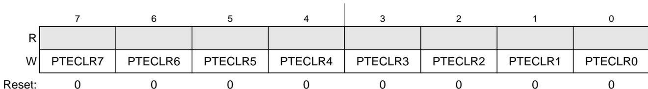
**Figure 6-29. Port E Data Clear Register (PTECLR)**
