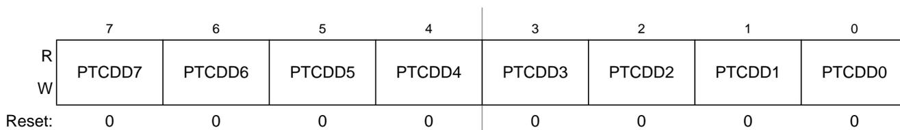
Figure 6-14. Port C Data Direction Register (PTCDD)
