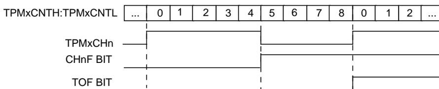
**Figure 16-3. High-True Pulse of an Edge-Aligned PWM**
