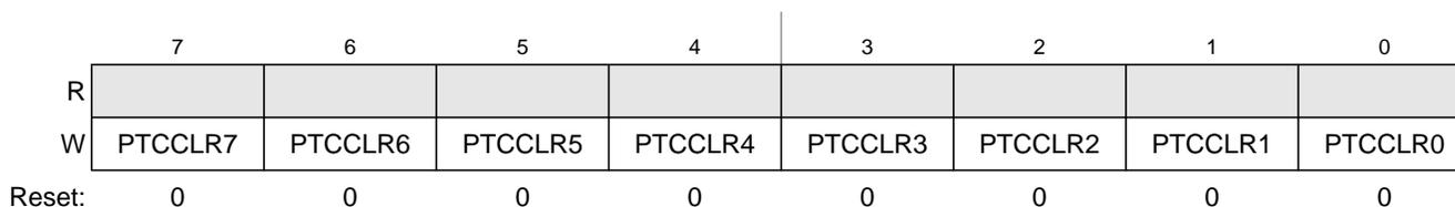
**Figure 6-16. Port C Data Clear Register (PTCCLR)**
