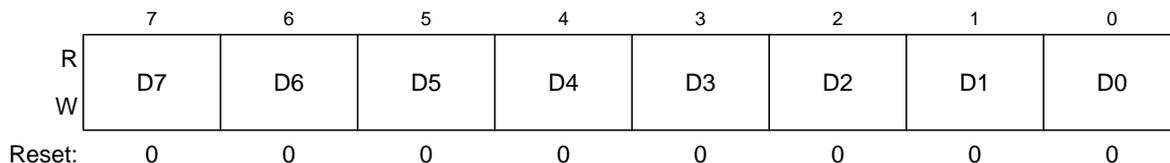
Figure 4-7. Linear Byte Post Increment Register (LBP)
