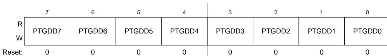
Figure 6-40. Port G Data Direction Register (PTGDD)
