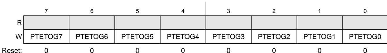
**Figure 6-30. Port E Toggle Register (PTETOG)**
