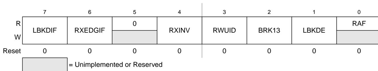
**Figure 14-10. SCI Status Register 2 (SCiXS2)**
