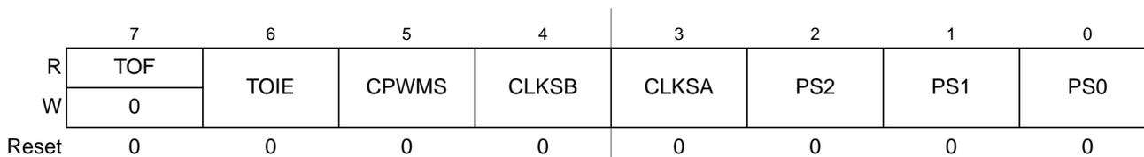
Figure 16-7. TPM Status and Control Register (TPMxSC)
