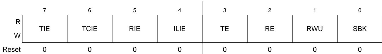
**Figure 14-8. SCI Control Register 2 (SC1xC2)**
