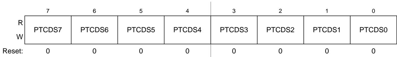
Figure 6-20. Drive Strength Selection for Port C Register (PTCDS)
