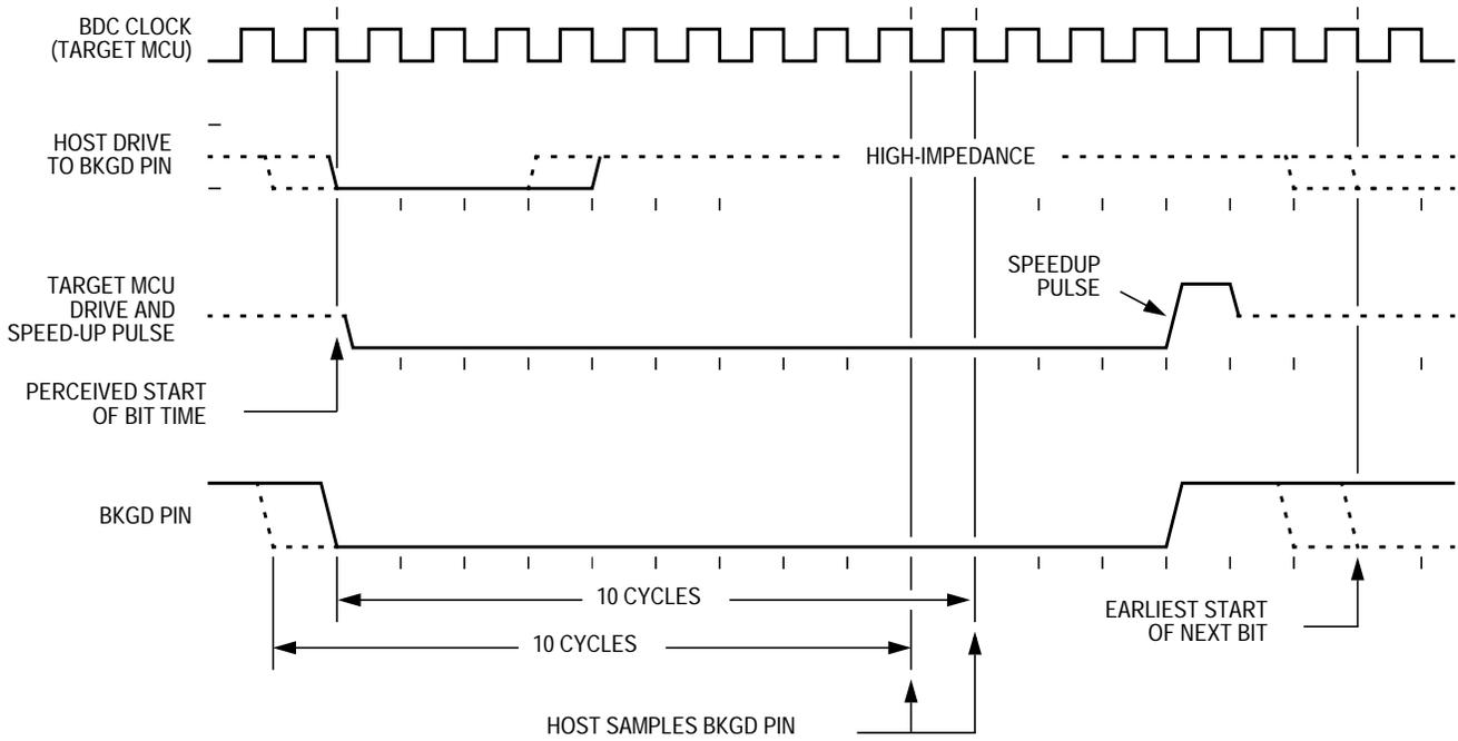
Figure 17-4. BDM Target-to-Host Serial Bit Timing (Logic 0)
