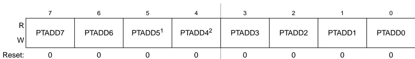
**Figure 6-4. Port A Data Direction Register (PTADD)**
