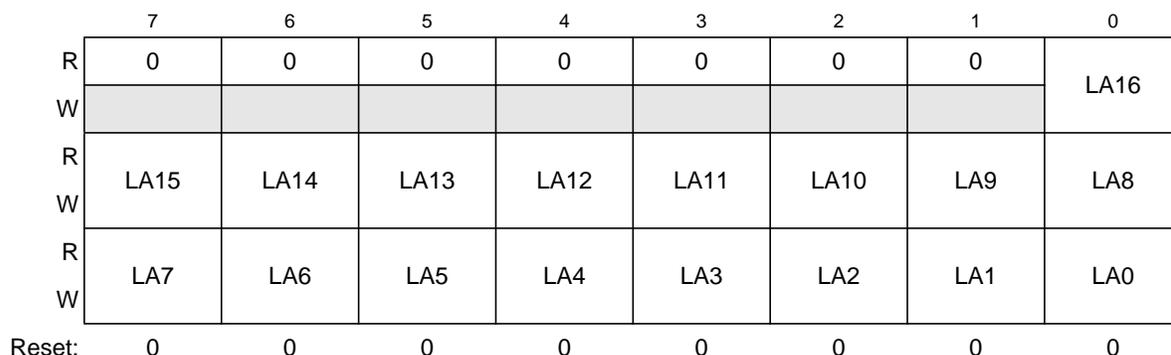
Figure 4-5. Linear Address Pointer Registers 2:0 (LAP2:LAP0)
