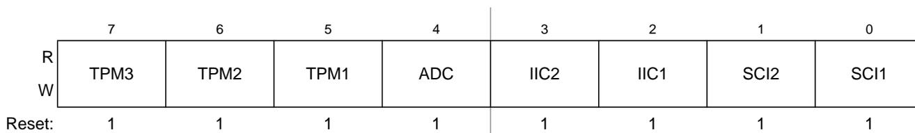
**Figure 5-12. System Clock Gating Control 1 Register (SCGC1)**
