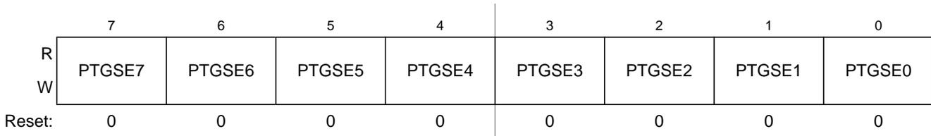
**Figure 6-42. Slew Rate Enable for Port G Register (PTGSE)**
