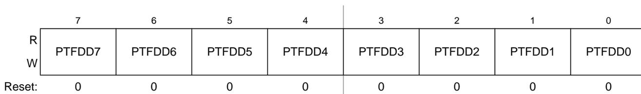
Figure 6-35. Port F Data Direction Register (PTFDD)
