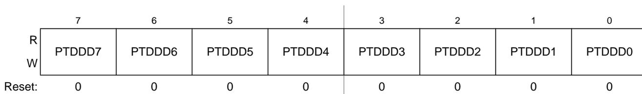
Figure 6-22. Port D Data Direction Register (PTDDD)
