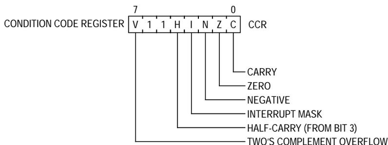
Figure 8-2. Condition Code Register
