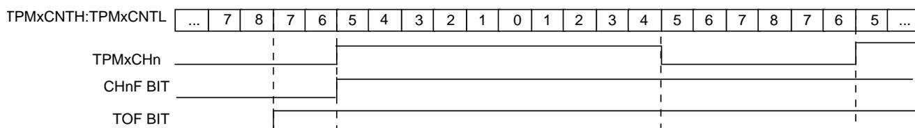
**Figure 16-5. High-True Pulse of a Center-Aligned PWM**
