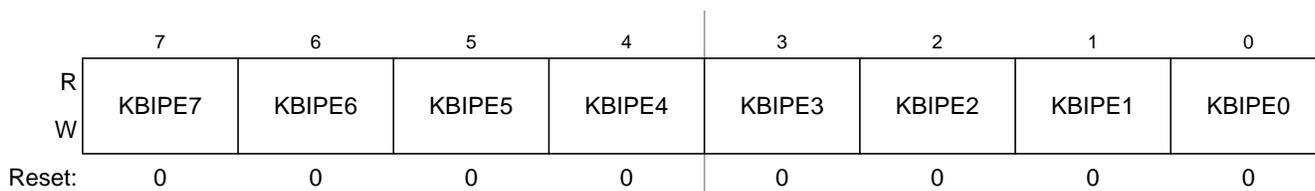
Figure 7-3. KBI Interrupt Pin Select Register (KBIXPE)
