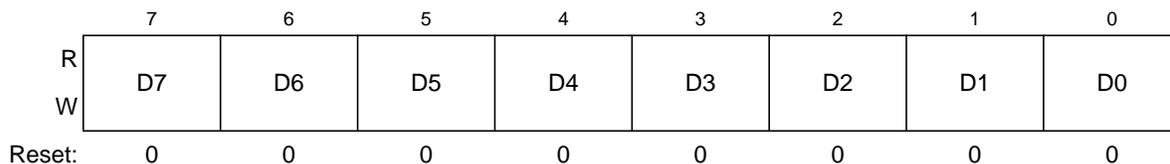
Figure 4-6. Linear Word Post Increment Register (LWP)
