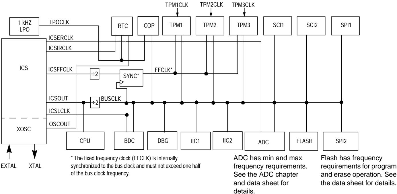
Figure 1-2. System Clock Distribution Diagram
