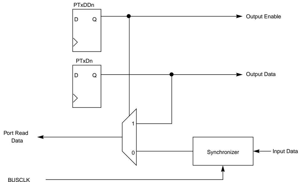
Figure 6-1. Parallel I/O Block Diagram
