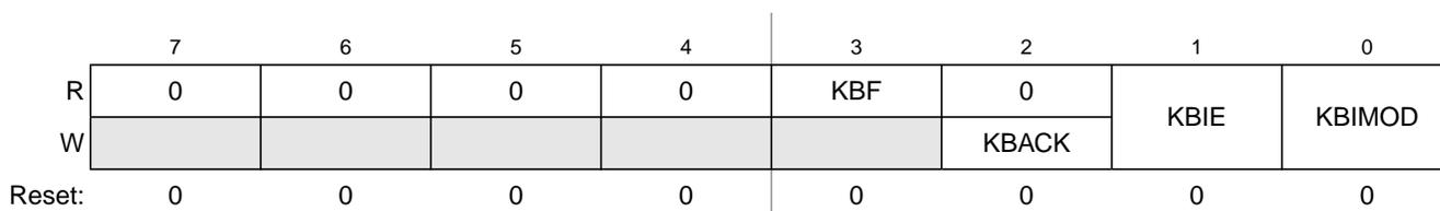
Figure 7-2. KBI Interrupt Status and Control Register (KBIXSC)
