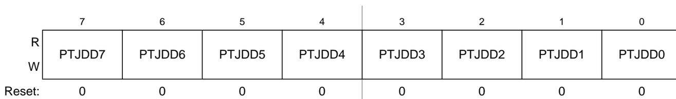
Figure 6-50. Port J Data Direction Register (PTJDD)
