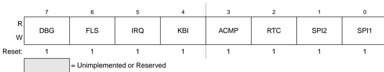
**Figure 5-13. System Clock Gating Control 2 Register (SCGC2)**
