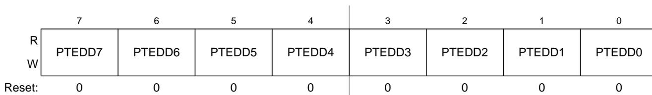
Figure 6-27. Port E Data Direction Register (PTEDD)
