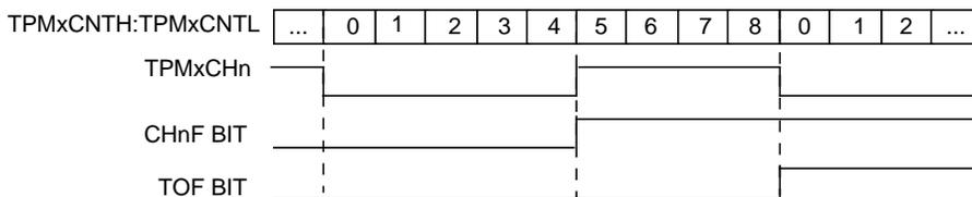
**Figure 16-4. Low-True Pulse of an Edge-Aligned PWM**
