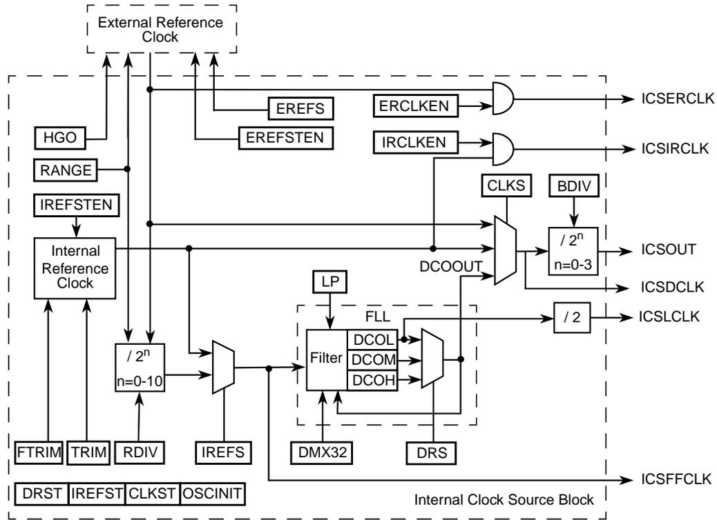
Figure 11-2. Internal Clock Source (ICS) Block Diagram
