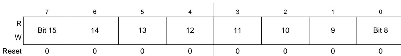
**Figure 16-13. TPM Channel Value Register High (TPMxCnVH)**
