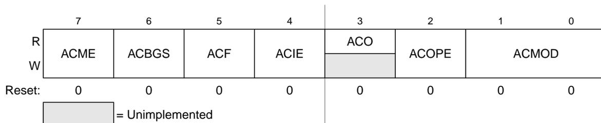
Figure 9-3. ACMPx Status and Control Register
