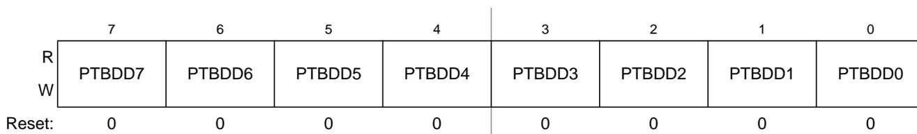
Figure 6-9. Port B Data Direction Register (PTBDD)
