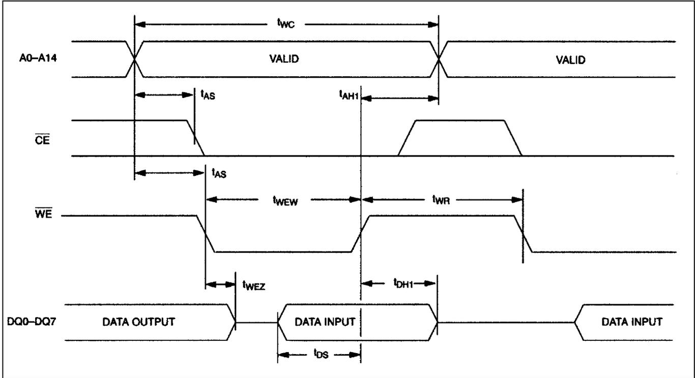
**WRITE CYCLE TIMING DIAGRAM, CHIP-ENABLE CONTROLLED**
