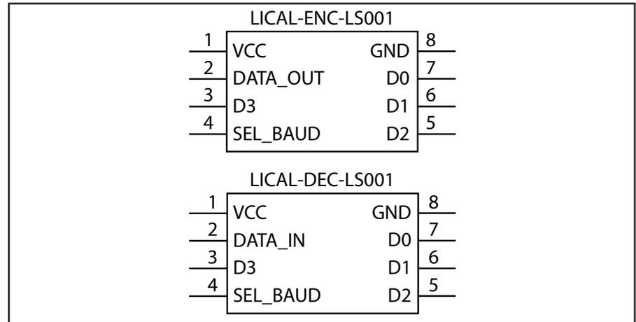
Figure 3: LS Series Encoder and Decoder Pin Assignments
