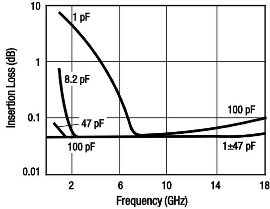
**Figure 1. Typical Insertion Loss vs Frequency
