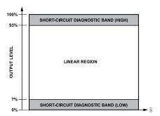
Figure 20. Short-Circuit Diagnostic Band
