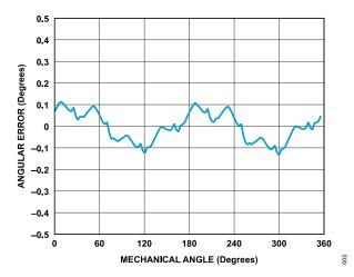
Figure 5. Angular Error vs. Mechanical Angle After Offset Correction
