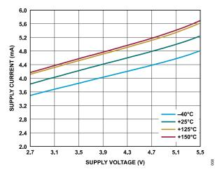
Figure 8. Supply Current vs. Supply Voltage
