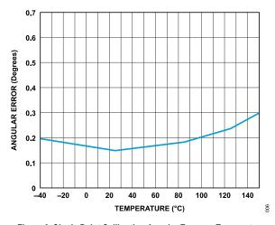
Figure 6. Single Point Calibration Angular Error vs. Temperature
