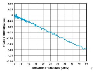
Figure 12. Phase Error vs. Mechanical RPM
