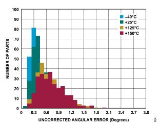
Figure 4. Uncorrected Angular Error Histogram
