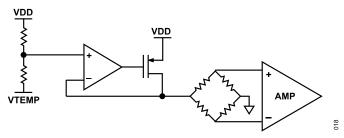
Figure 17. Temperature Compensated Bridge Driver
