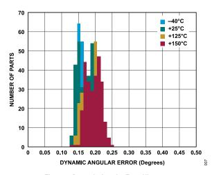
Figure 7. Dynamic Angular Error Histogram
