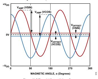
Figure 15. Differential Output Voltage Range
