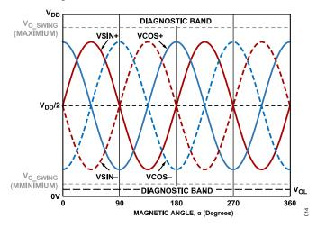
Figure 14. Single-Ended Output Voltage Range
