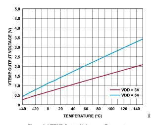
Figure 9. VTEMP Output Voltage vs. Temperature
