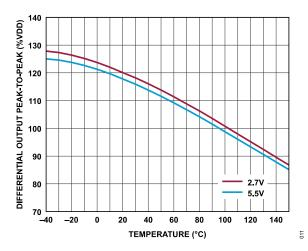
Figure 11. Differential Output Peak-to-Peak vs. Temperature
