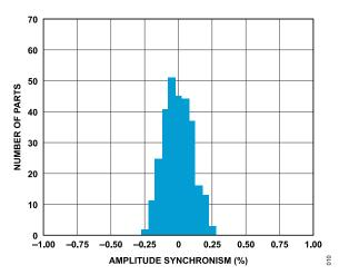
Figure 10. Amplitude Synchronism Histogram
