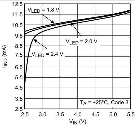
Figure 17. Indicator Current vs Input Voltage VLED
