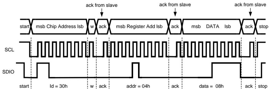
w = write (SDA = 0); ack = acknowledge (SDA pulled down by the slave): id = chip address, 30h for LM3555
