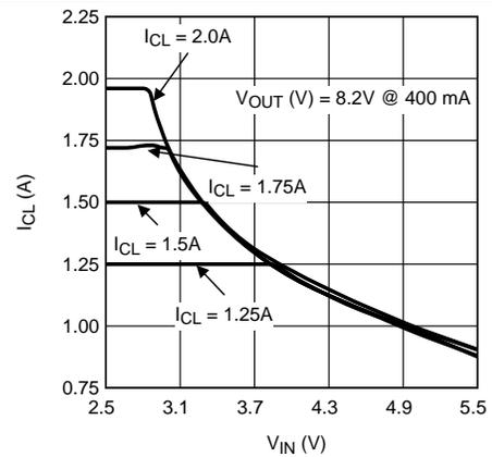
Figure 18. Inductor Current Limit vs Input Voltage
