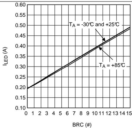
Figure 9. Single LED Flash Current vs Brightness Code
