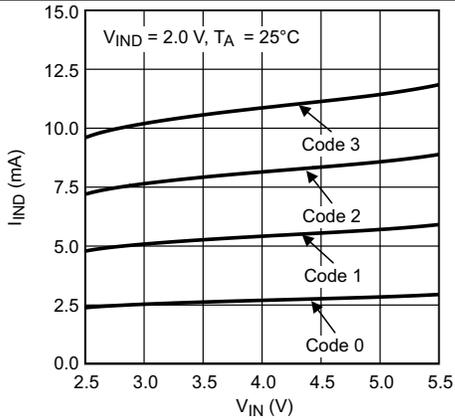
Figure 15. Indicator Current vs Input Voltage Brightness Codes
