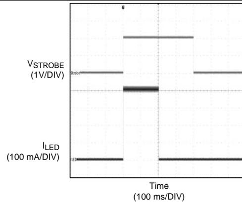
**Figure 38. Level Sensitive Strobe With Timeout**
