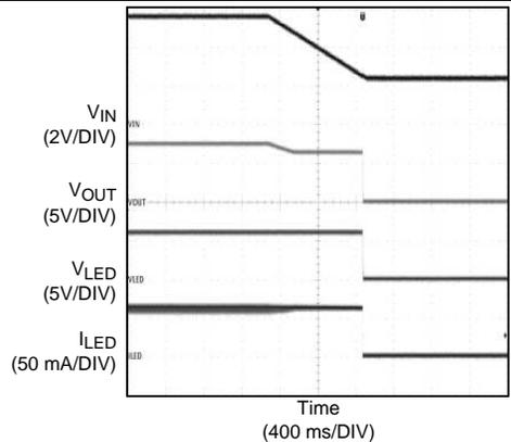
**Figure 35. Undervoltage Lockout (UVLO)**
