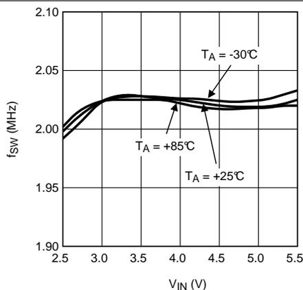
Figure 23. Frequency vs Input Voltage
