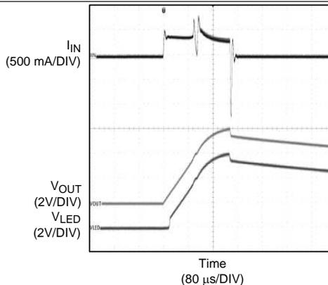
**Figure 34. Broken Inductor Fault**
