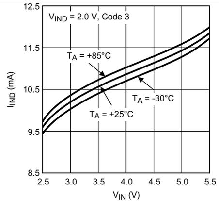
Figure 16. Indicator Current vs Input Voltage Tri-Temp
