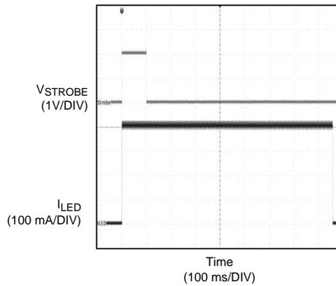
**Figure 39. Level Sensitive Strobe Without Timeout**
