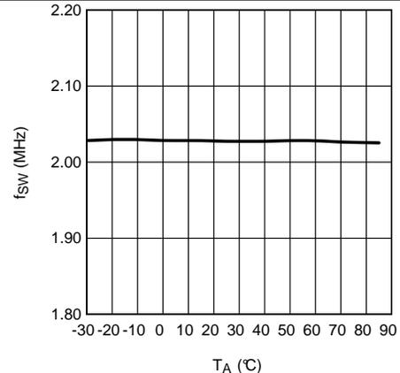
Figure 22. Frequency vs Temperature
