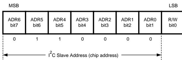
Figure 44. Device Address
