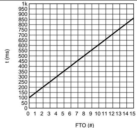
Figure 24. Flash Timeout Time vs Flash Timeout Code
