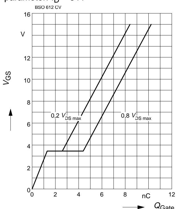
**Typ. gate charge (P-Ch.)** $V_{GS} = f(Q_{Gate})$ parameter:  $I_D = -2 \text{ A}$
