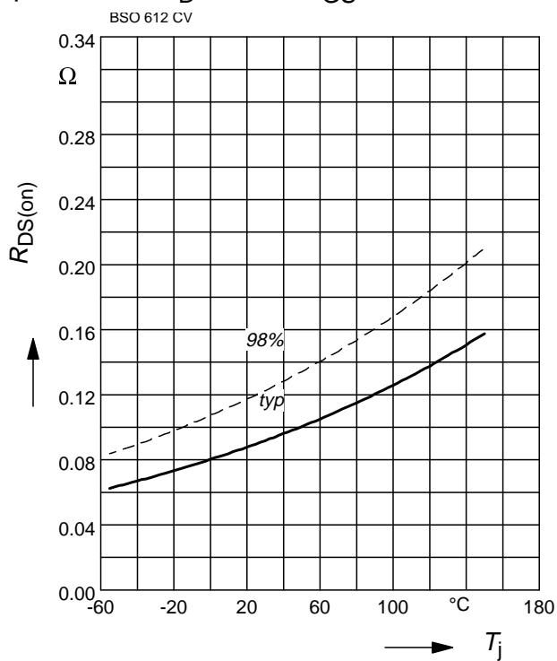
**Drain-source on-resistance (P-Ch.)**
