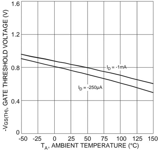
Fig. 19 Gate Threshold Variation vs. Ambient Temperature
