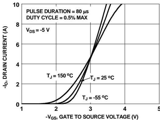
**Figure 5. Transfer Characteristics**
