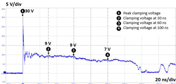
**Figure 5. ESD response to IEC 61000-4-2 (-8 kV contact discharge)**
