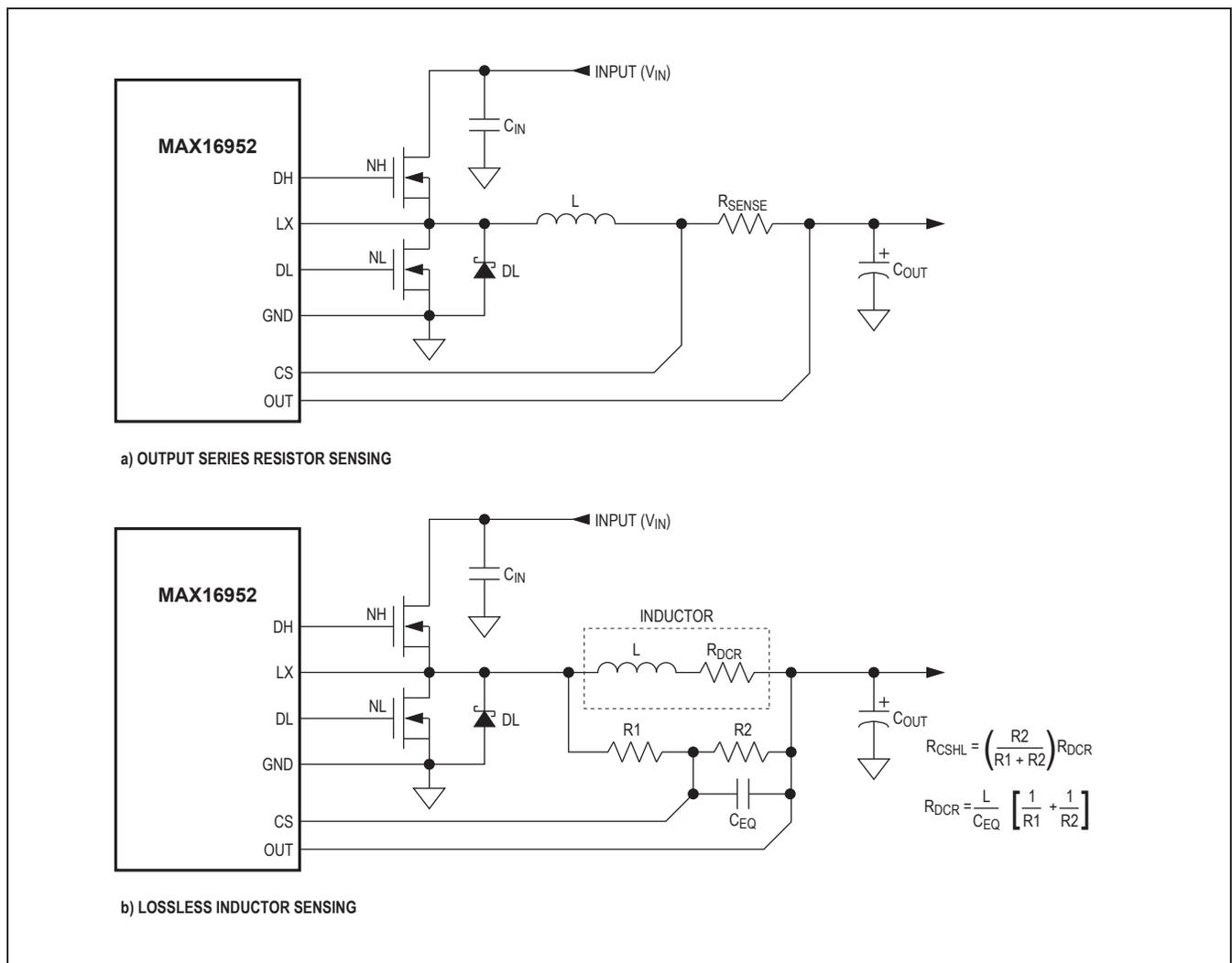
Figure 4. Current-Sense Configurations
