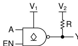
**Figure 6. Gated Voltage Translating Inverter Schematic Using SN74LVC1G38**
