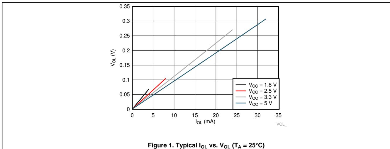
Figure 1. Typical  $I_{OL}$  vs.  $V_{OL}$  ( $T_A = 25^\circ\text{C}$ )
