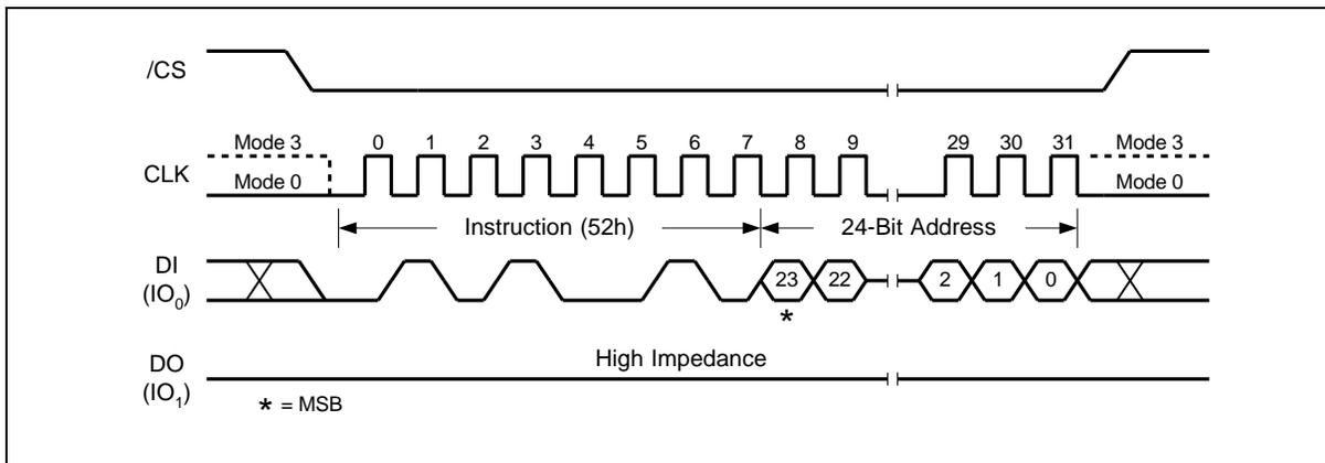
Figure 22a. 32KB Block Erase Instruction Sequence Diagram
