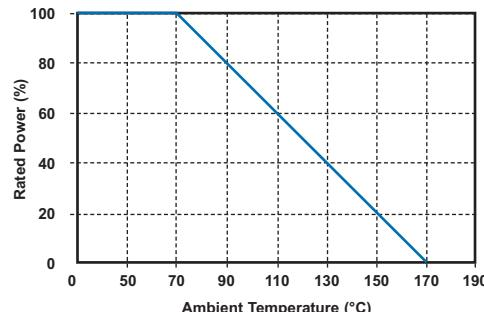
For resistors operated in ambient temperatures above 70°C, power rating must be derated in accordance with this curve.
