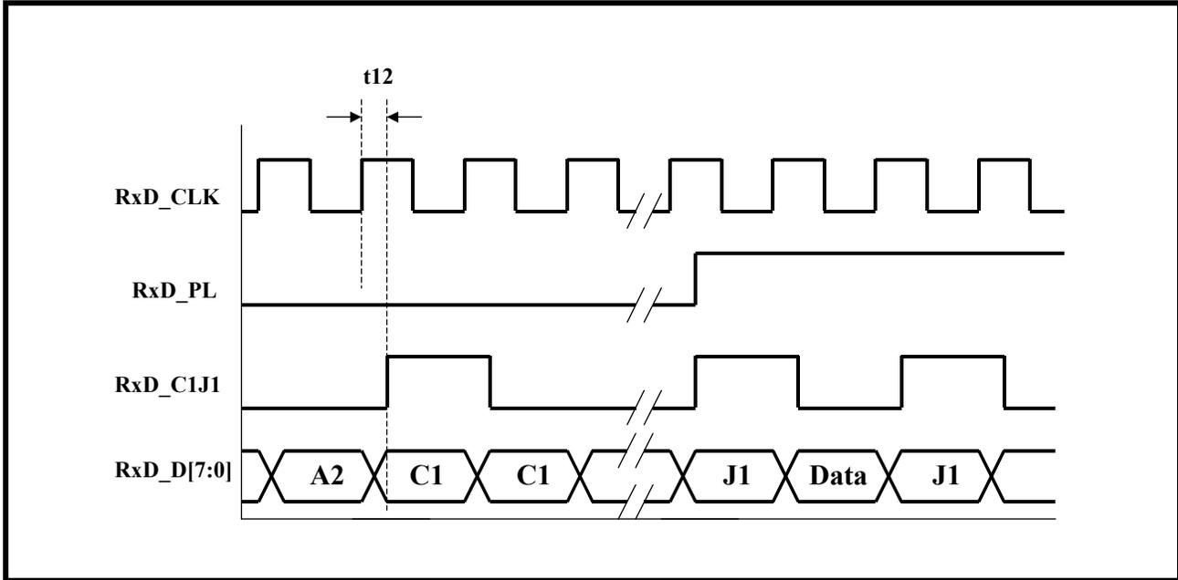
Table 20 presents information on the Timing Parameters for the Receive STS-1/STM-0 Telecom Bus Interface (when configured to operate in the STS-3/STM-1 Mode).
