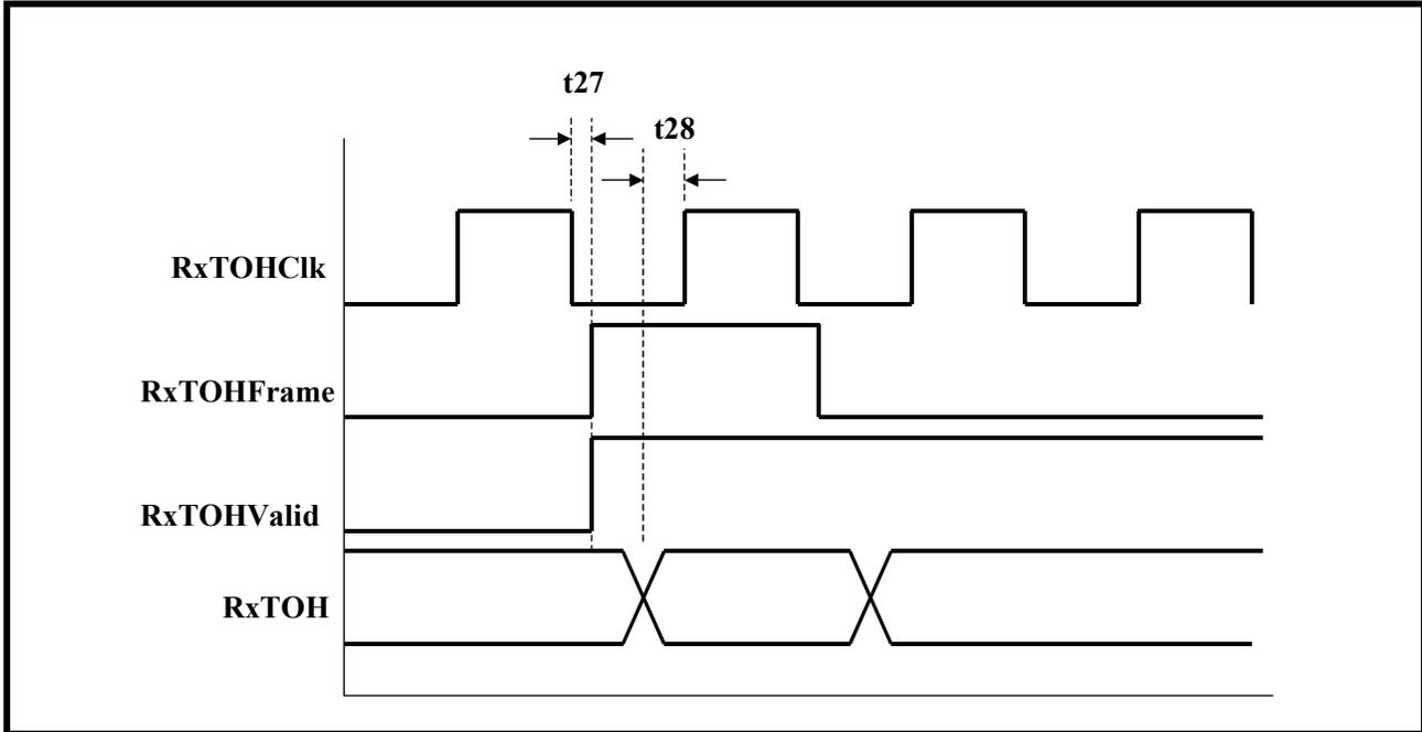
NOTE: The values for  $t_{27}$  and  $t_{28}$  can be found in [Table 28](#).
