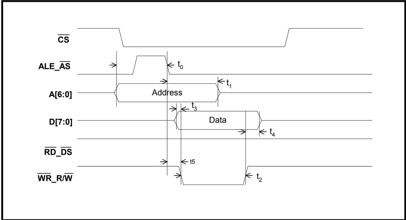
**NOTE:** The values for  $t_0$  through  $t_7$ , within this figure can be found in [Table 3](#).
