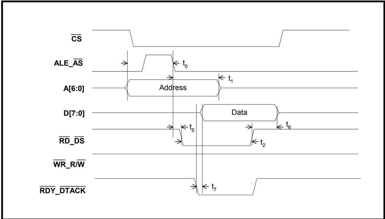
**NOTE:** The values for  $t_0$  through  $t_7$ , within this figure can be found in [Table 3](#).
