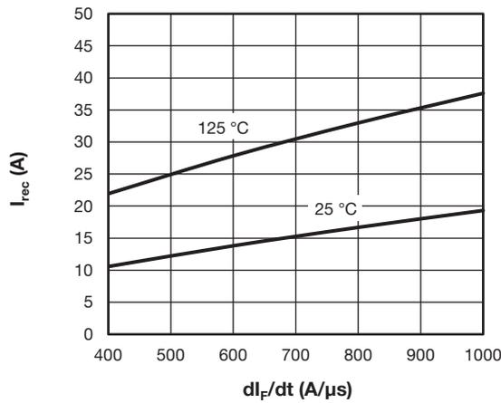
Fig. 9 - Typical Reverse Recovery vs.  $di_F/dt$
