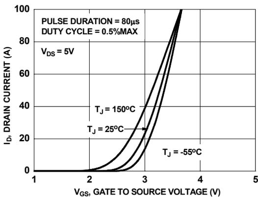
**Figure 5. Transfer Characteristics**
