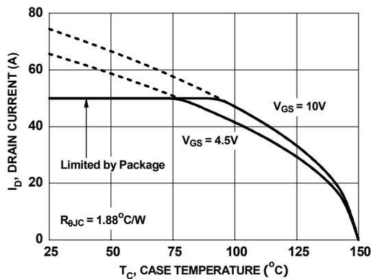
**Figure 11. Maximum Continuous Drain Current vs Ambient Temperature**
