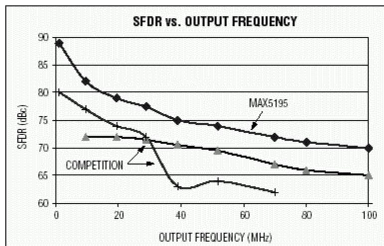
Figure 1. This SFDR graph compares the MAX5195 to the best available competitive devices for a range of output frequencies.
