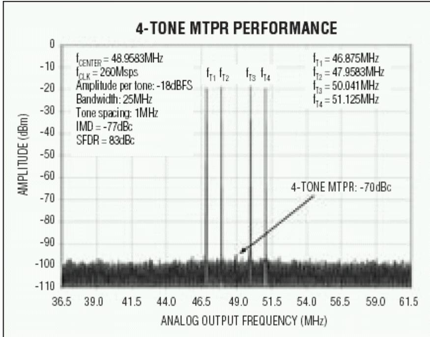
Figure 6. This four-carrier test-vector spectral plot illustrates the MAX5195's superior multitone IMD performance for GSM applications. The output frequency is centered at 48MHz.
