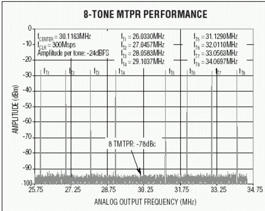
Figure 5. This eight-carrier test-vector spectral plot illustrates the MAX5888's superior multitone IMD performance for CDMA applications. The selected output frequency is centered at 30MHz.
