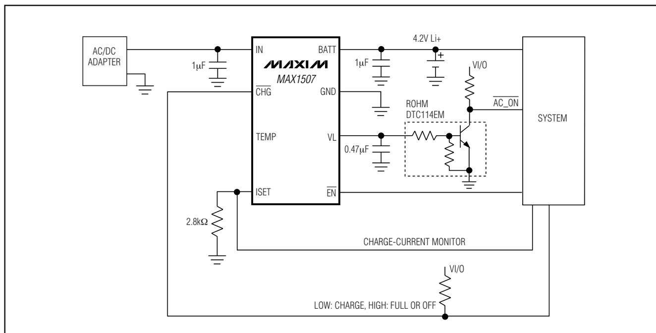
Figure 3.  $\mu$ P Interfaced Li+ Battery Charger
