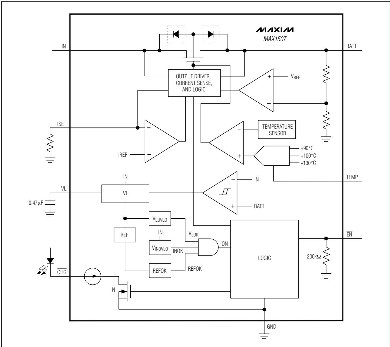
Figure 1. Functional Diagram
