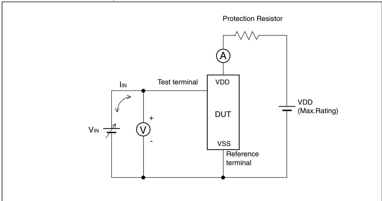
Note : The voltage  $V_{\text{IN}}$  is increased gradually and the current  $I_{\text{IN}}$  of 300 mA at maximum shall flow.
