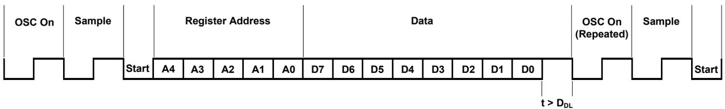
To concatenate write operations, repeat Osc On, Sample and Start after the DO bit of the previous sequence as shown.
