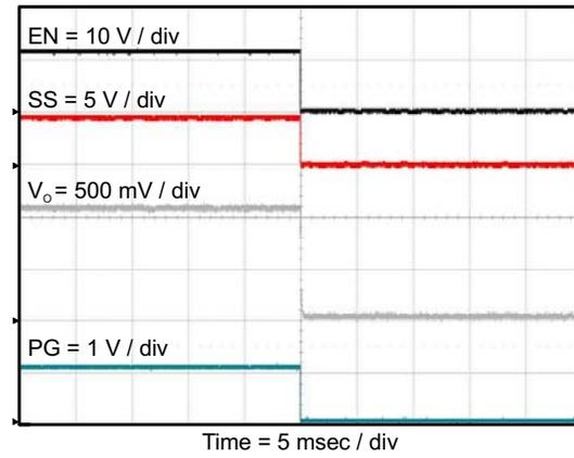
**Figure 42. TPS563219 Shut Down Relative To EN**
