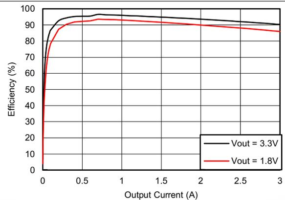
Figure 14. Efficiency vs Output Current (V<sub>I</sub> = 5V)
