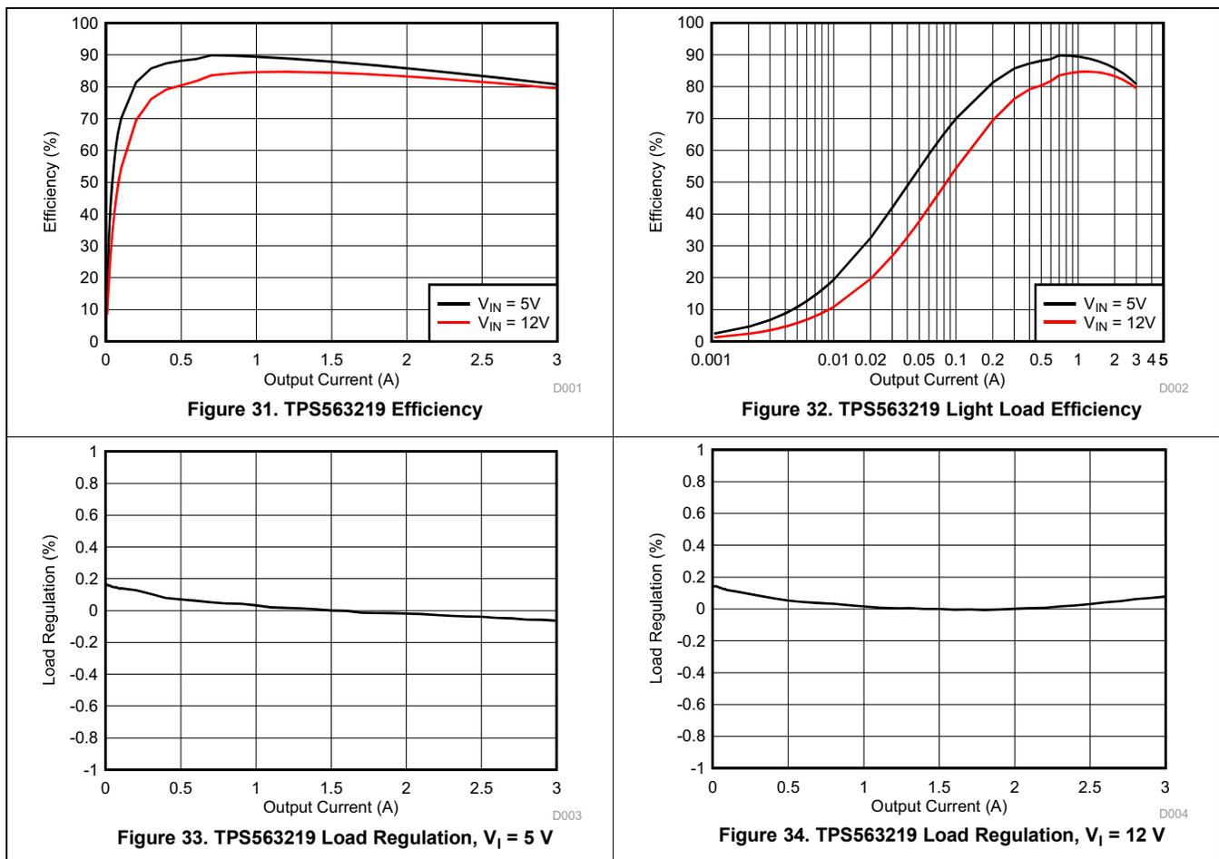
The following application curves were generated using the application circuit of [Figure 30](#).
