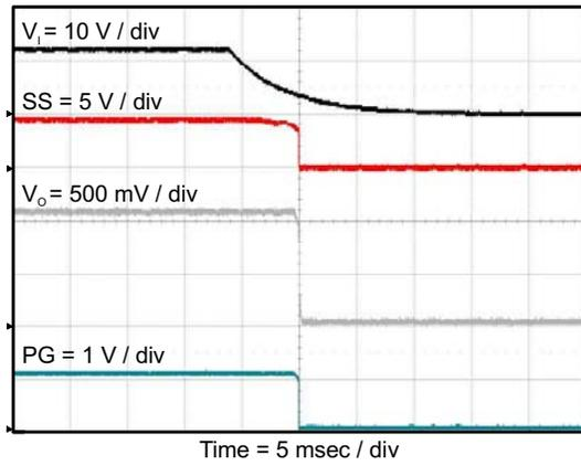
**Figure 41. TPS563219 Shut Down Relative To  $V_i$**
