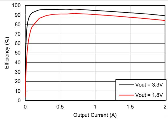
**Figure 6. Efficiency vs Output Current (V<sub>I</sub> = 5V)**
