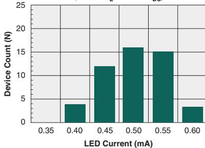
Typical I<sub>F</sub> for Switch Dropout
