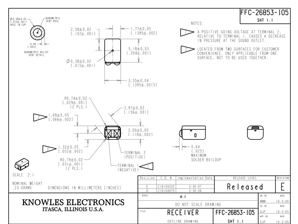
THE FFC-26853-105 IS A FERROFLUID DAMPED AND EXTERNALLY VENTED FC-26171-000 RECEIVER WITH A PEAK OF 5dB RELATIVE TO THE SENSITIVITY AT IKHZ UNDER CONSTANT VOLTAGE DRIVE CONDITIONS.
