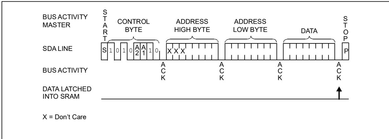
**FIGURE 4-5: SRAM SEQUENTIAL WRITE**
