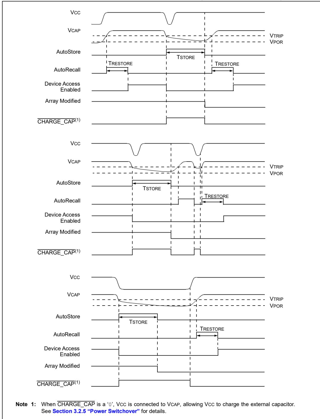
FIGURE 3-3: AUTOSTORE/AUTORECALL SCENARIOS (WITH ARRAY NOT MODIFIED)
