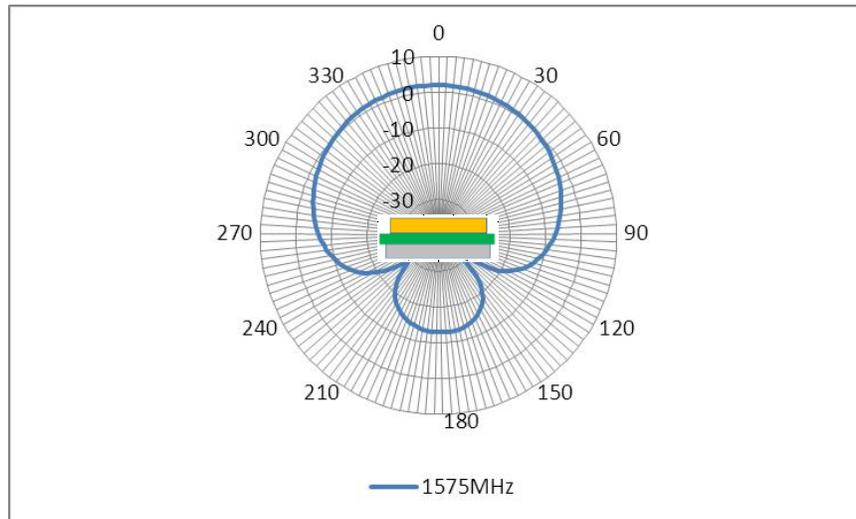
RHCP Radiation Pattern (70mm x 70mm ground plane ) GLONASS
