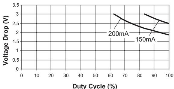
**Device Duty Cycle vs.  $V_{DROD}$**
