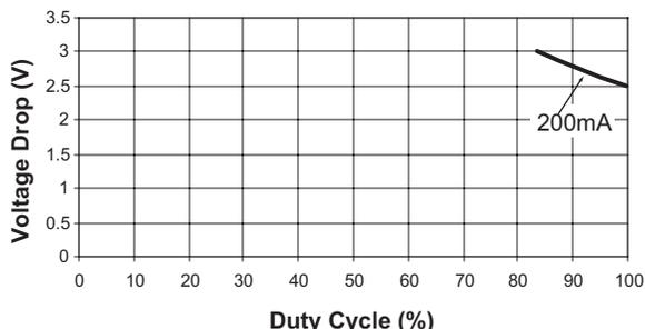
**Device Duty Cycle vs.  $V_{DROD}$**
