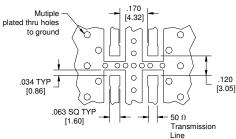
Dimensions are in Inches [Millimeters] JP506S Mounting Footprint
