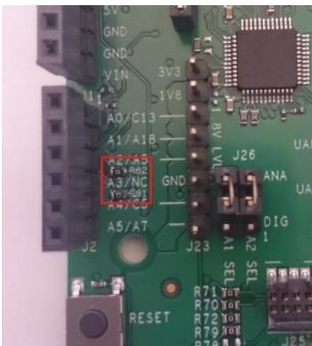
Figure 8: Resistors R81 and R82
