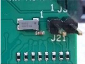
Figure 9: 32.768 kHz oscillator and pin header J21
