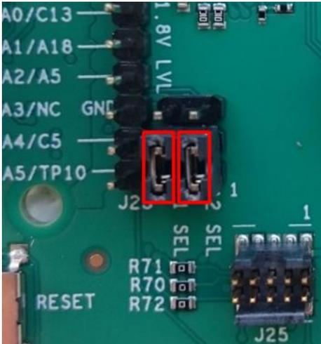
Figure 7: A1 and A2 as digital I/O on J2
