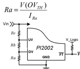
**Figure 17:** UV & OV three-resistor divider configuration.
