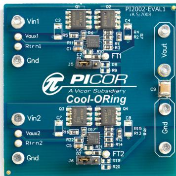
**Figure 24:** PI2002 Mounted on PI2002-EVAL1
