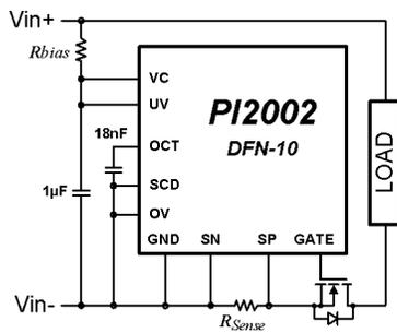
**Figure 22:** PI2002 (10L-TDFN package) in low side disconnect switch application
