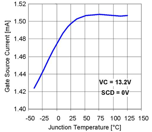
Figure 15: Gate output source current vs. temperature
