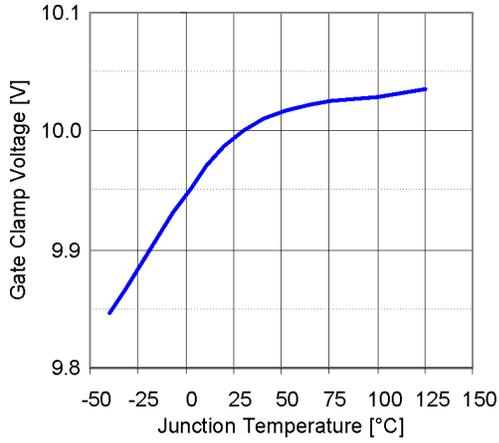
Figure 14: Gate to SP clamp voltage vs. temperature.
