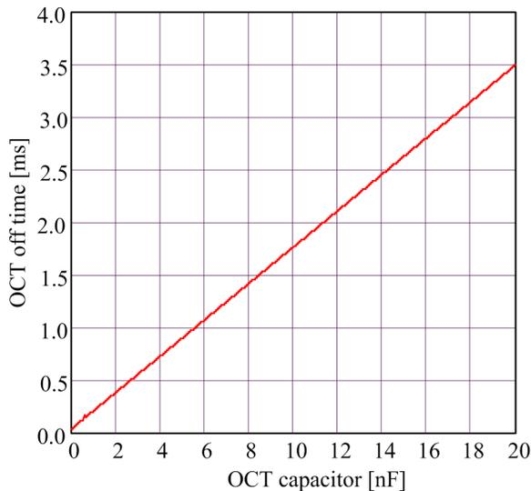
**Figure 3:** OCT Off time vs. OCT capacitor value
