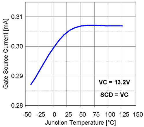
Figure 16: Gate output source current vs. temperature
