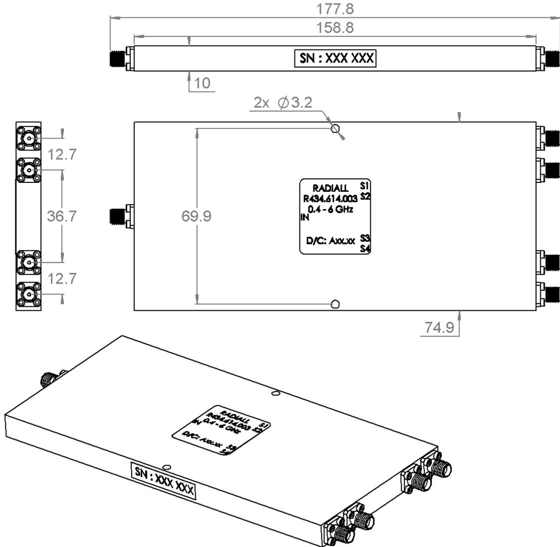
All dimensions are in mm. Tolerances according ISO 2768 m-K
