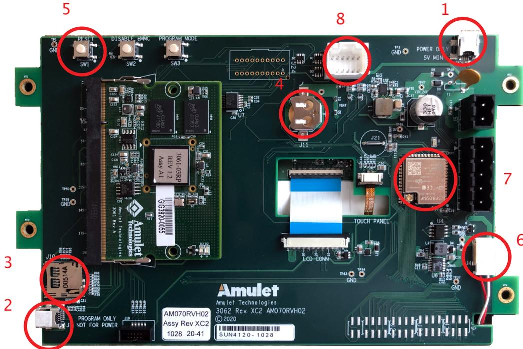
1. Mini-USB input power supply: This port designated J18 on the PCB is just one of many methods to power the display module. The power supply must be  $5V \pm 5\%$ , supplying at least 1A.
