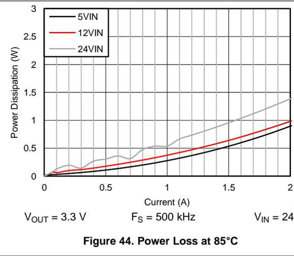
Figure 44. Power Loss at 85°C
