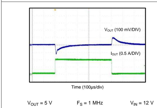
**Figure 61. Load Transient 0.1 A to 1 A**
