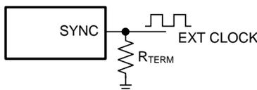
Figure 32. Frequency Synchronization
