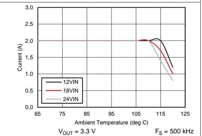
Figure 50. Derating Curve
