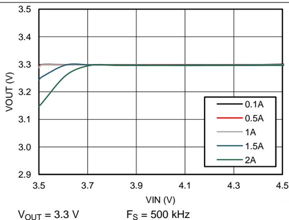
Figure 9. Dropout Curve
