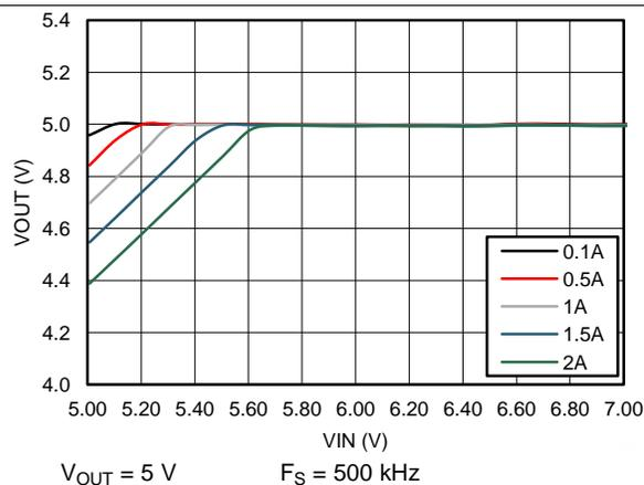
Figure 10. Dropout Curve
