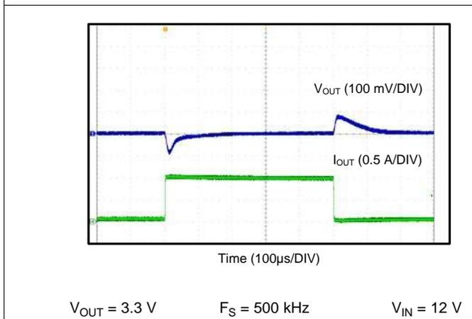
Figure 49. Load Transient
