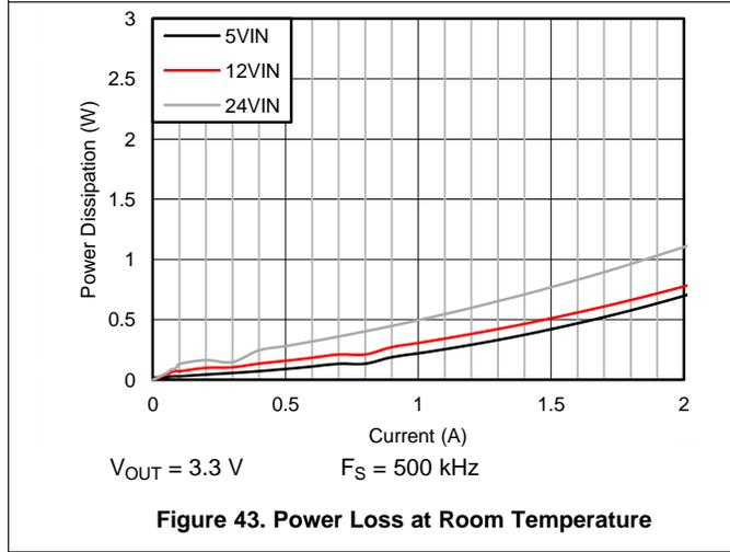
Figure 43. Power Loss at Room Temperature
