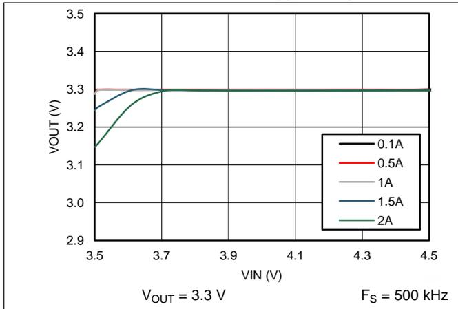
Figure 45. Dropout Voltage
