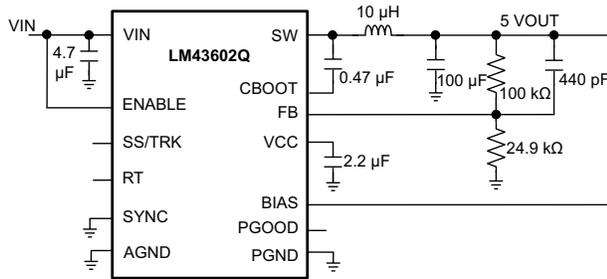
$V_{OUT} = 5\text{ V}$   $F_S = 500\text{ kHz}$
