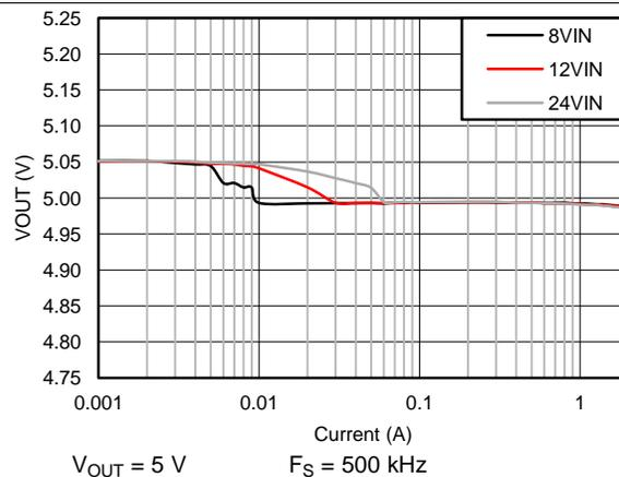
Figure 8.  $V_{OUT}$  Regulation
