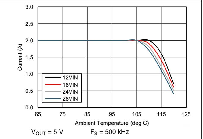
**Figure 62. Derating Curve**
