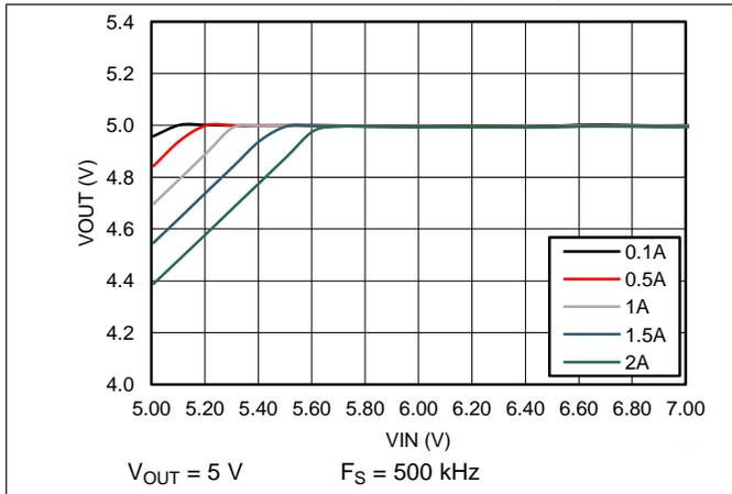
**Figure 57. Dropout Voltage**
