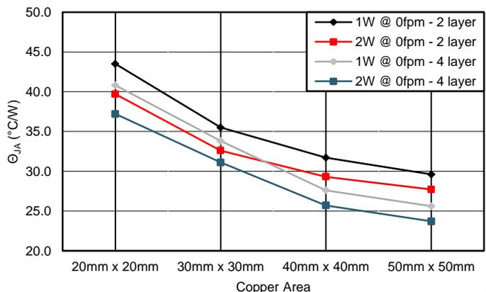
Figure 64.  $R_{\theta JA}$  vs Copper Area
