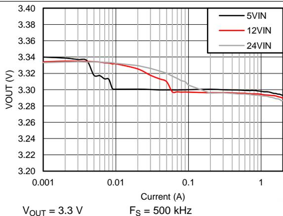
Figure 7.  $V_{OUT}$  Regulation
