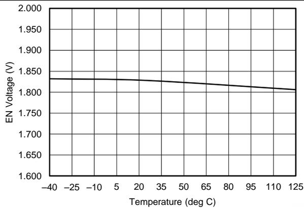
**Figure 13. EN Falling Threshold vs Junction Temperature**
