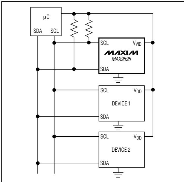
Figure 6. Typical I<sup>2</sup>C Interface Application
