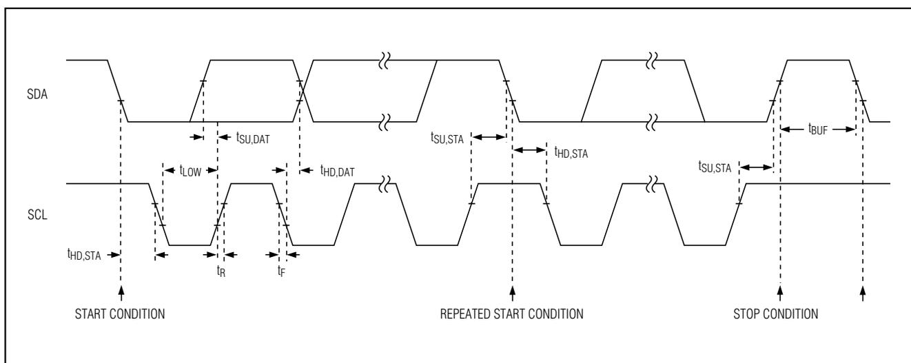
Figure 5. SDA and SCL Signal Timing Diagram
