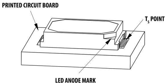
$T_S$  can be easily measured by mounting a thermocouple on the soldering joint as shown in preceding figure, while  $R_{\theta J-S}$  is provided in the data sheet. Verify the  $T_S$  of the LED in the final product to ensure that the LEDs are operating within all maximum ratings stated in the data sheet.
