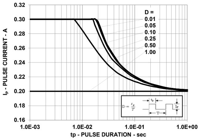
Figure 16: Pulse Handling Capability at  $T_s = 100^\circ\text{C}$  (Royal Blue)
