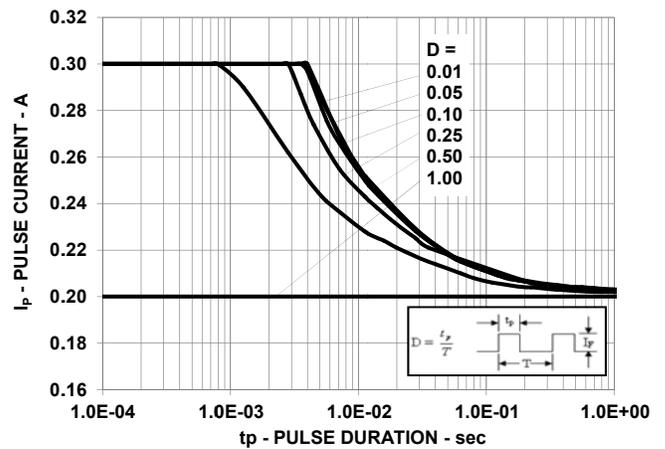
Figure 15: Pulse Handling Capability at  $T_s \leq 98^\circ\text{C}$  (Royal Blue)
