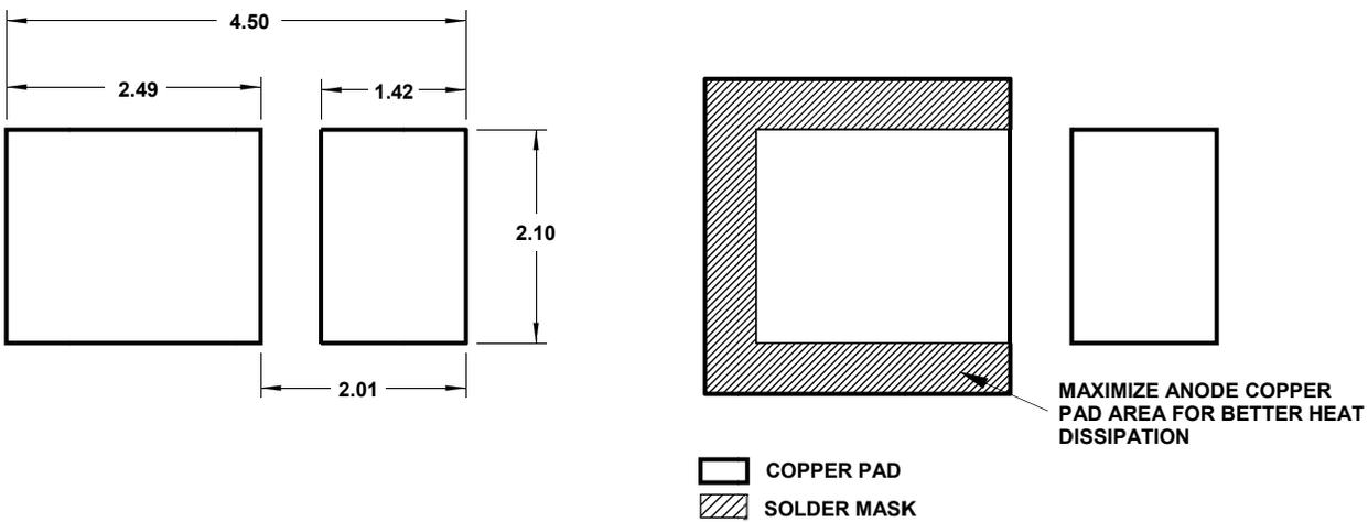
NOTE: All dimensions are in millimeters (mm).
