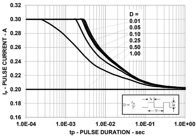
Figure 14: Pulse Handling Capability at T<sub>s</sub> ≤ 100°C (Far Red)
