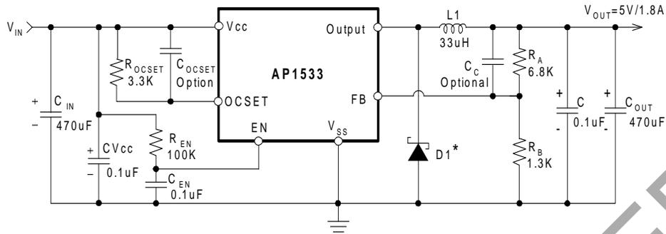
$$V_{OUT} = V_{FB} \times (1 + R_A/R_B)$$
