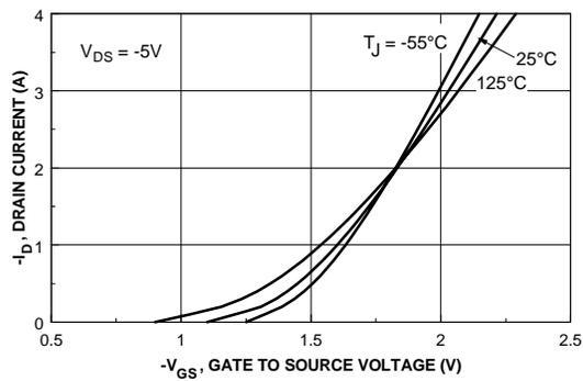
Figure 5. Transfer Characteristics.
