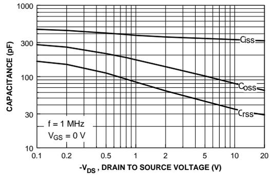
Figure 8. Capacitance Characteristics.
