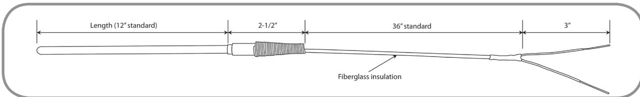
*Thermocouple calibration type N is available in all sizes.*
