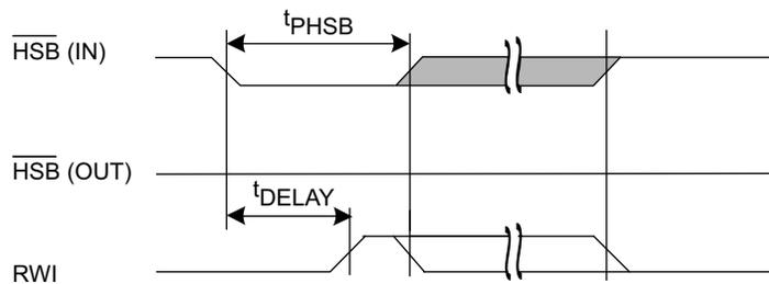
HSB pin is driven HIGH to  $V_{CC}$  only by Internal 100 K $\Omega$  resistor, HSB driver is disabled
