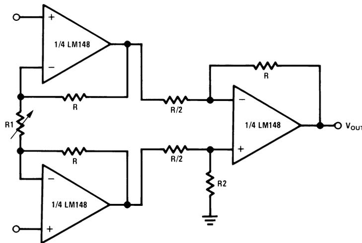
$$V_{OUT} = 2 \left( \frac{2R}{R1} + 1 \right), V_S - 3V \leq V_{IN CM} \leq V_S + - 3V,$$
