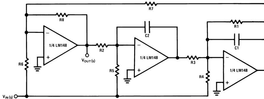
$$Q = \sqrt{\frac{R8}{R7}} \times \frac{R1C1}{\sqrt{R3C2R2C1}}, f_0 = \frac{1}{2\pi} \sqrt{\frac{R8}{R7}} \times \frac{1}{\sqrt{R2R3C1C2}}, f_{\text{NOTCH}} = \frac{1}{2\pi} \sqrt{\frac{R6}{R3R5R7C1C2}}$$
