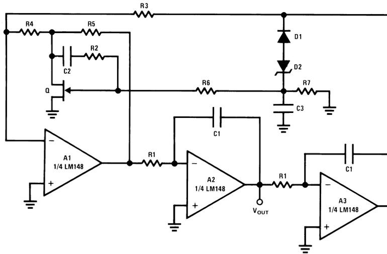
$$f = \frac{1}{2\pi R1 C1} \times \sqrt{K}, K = \frac{R4 R5}{R3} \left( \frac{1}{r_{DS}} + \frac{1}{R4} + \frac{1}{R5} \right), r_{DS} \approx \frac{R_{ON}}{\left( 1 - \frac{V_{GS}}{V_P} \right)^{1/2}}$$
