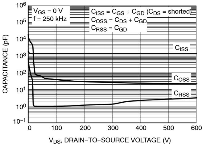
Figure 5. Capacitance Characteristics
