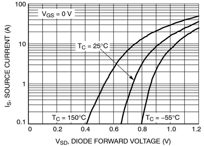
Figure 4. Diode Forward Voltage vs. Source Current
