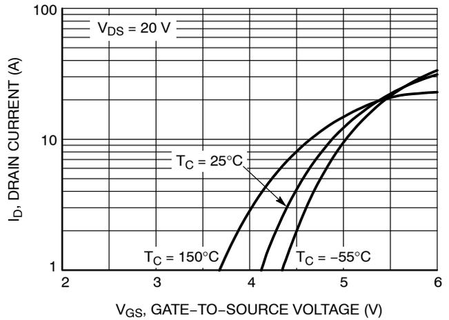
Figure 2. Transfer Characteristics
