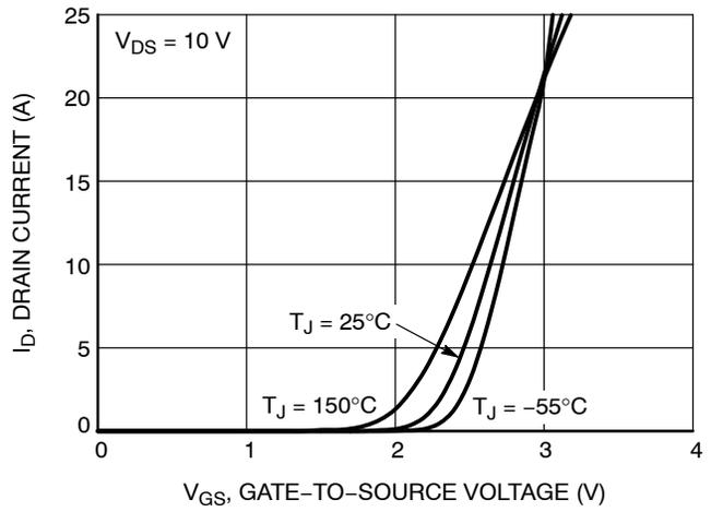
Figure 2. Transfer Characteristics
