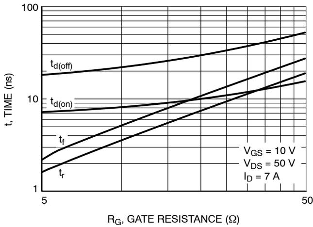
Figure 9. Resistive Switching Time Variation vs. Gate Resistance
